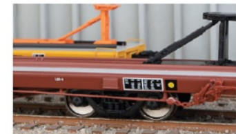
70-TON TRUCKS WITH 33" RP-25 METAL WHEELS
