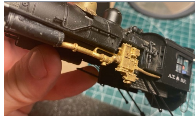
9. I added the feedwater heater to the fireman's side. The part fit perfectly in the section of running board where the original air compressor was mounted. Adding a few extra droplets of CA on top of the part once I mounted it allowed extra glue to flow into the cracks and crevices I couldn't see or access easily, further affixing it to the boiler shell.
