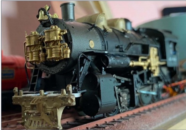
14. I added a small, cone-funneled dynamo above the smoke box and a bell from a Spectrum Russian 2-10-0.
