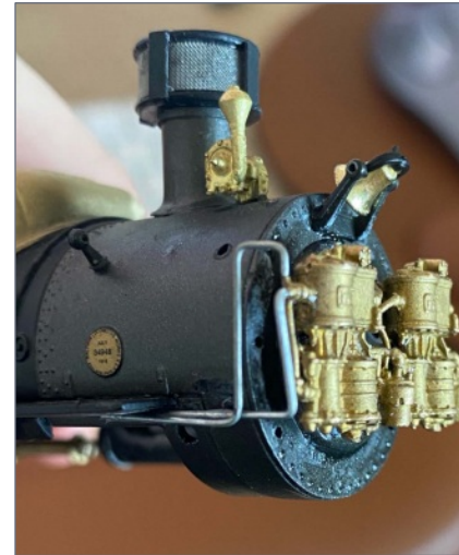
23. The last photo taken before moving, showing the wire I glued to the compressor.
