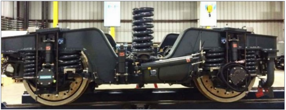
42a. Siemens-Mobility SF4 two-axle two-motor truck.
