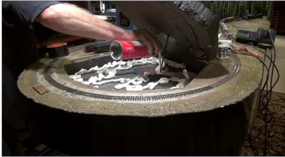
8. The assembled and tested turntable section is glued into the layout with sprayfoam adhesive.
