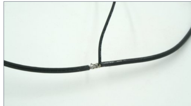
8. A soldered feeder connection.
