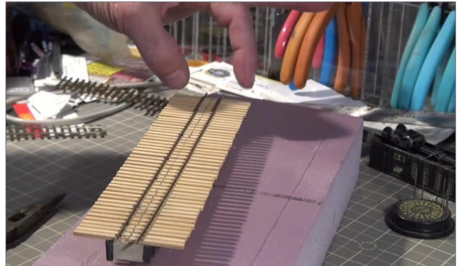
6. Ken assembles the turntable bridge by gluing ties to the top, and then hand-spiking the rails to the ties.
