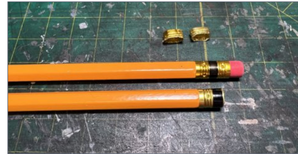
5. I cut off the ferrule from a standard pencil to create the water troughs.
