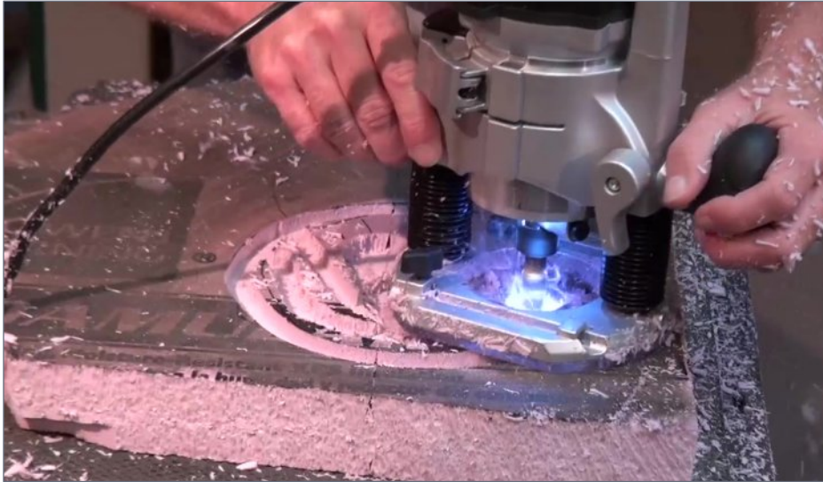
4. After drawing the center and outside circles for the turntable, Ken routs the turntable pit in the foam.
