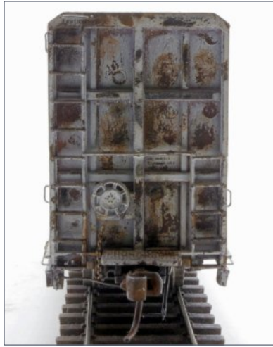
17. Head-on B-end view. Note the several added brass details. Uncoupling lever, see-through crossover platform, brake chain with brake bell crank that the chain curves 90°, grab irons, and a rubber air hose with angle cock.
