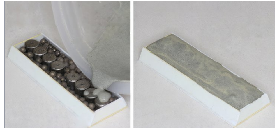
10. I made a custom tungsten weight the same size as the Tsunami decoder and placed it in the boiler where the Tsunami decoder would go.
