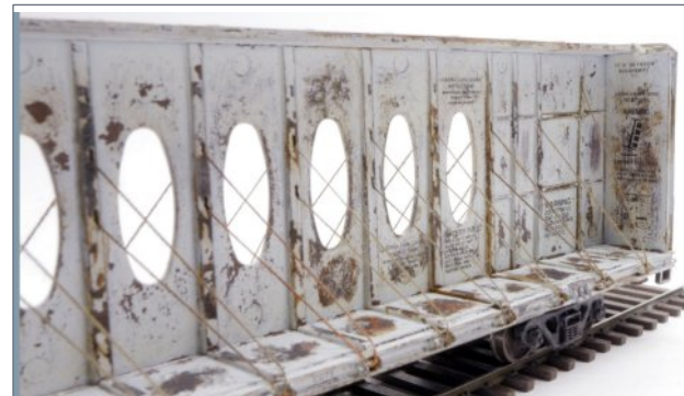
20. A-end view. The custom-made grab irons look much better than the original flush molded-on ones.
