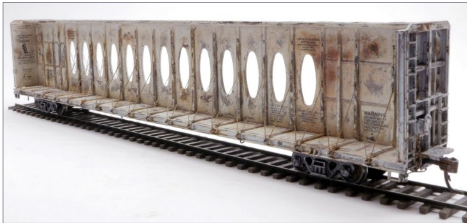
18. Left side view. I think the custom-made coupler lift bars add a little something to the car's overall look. The crossover platforms hide the long coupler shanks nicely. The long couplers allow the car to negotiate 22" curves without problem. I don't build or test for anything tighter.
