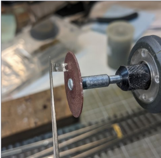
11. Trimmed the tab back using a rotary tool cutoff disk as a mini-grinder.
