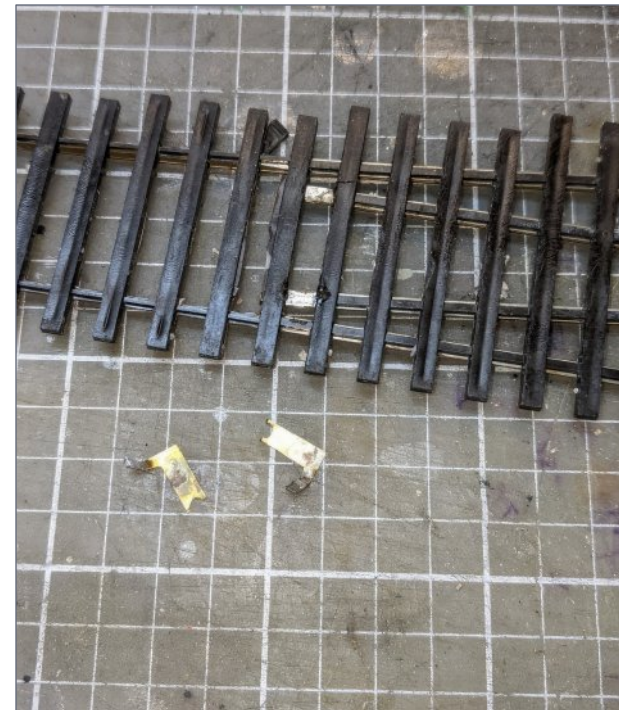
16. Here the brass strip has been removed (I cut it in half to make removal easier). I've also removed the plastic spacers between the ties [15] and will be taking a file to the bottom of the bare rail to smooth out any excess solder on the base of the rail.
