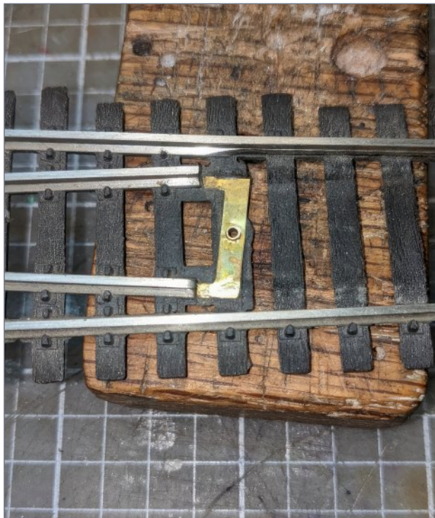
14. Remove the rivet and this brass strip at the end of the closure rails. See text for details.
