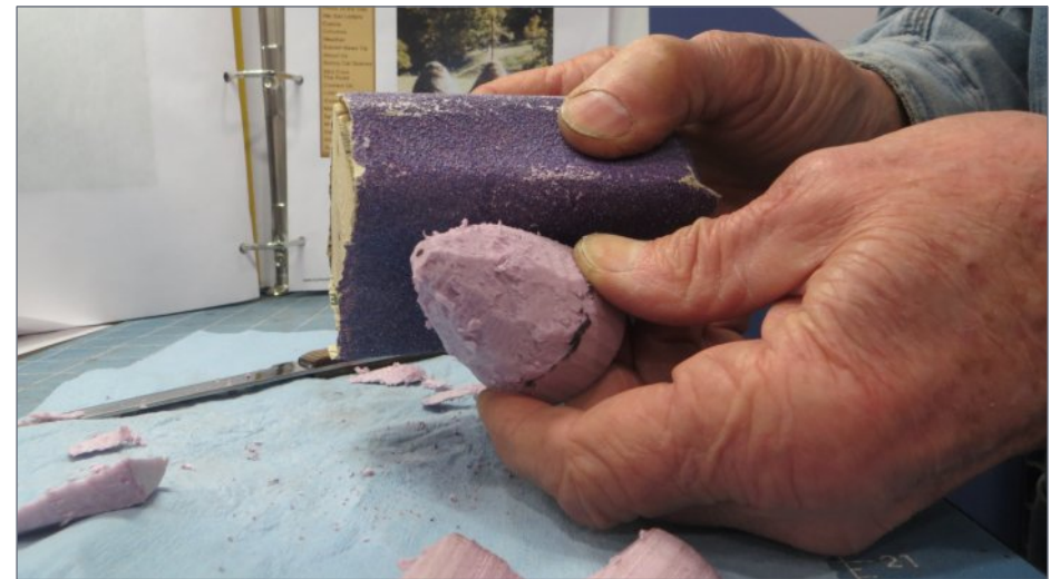
5. 80-grit sandpaper on a block made very quick work of yielding a nice, smooth finished shape to the foam forms.
