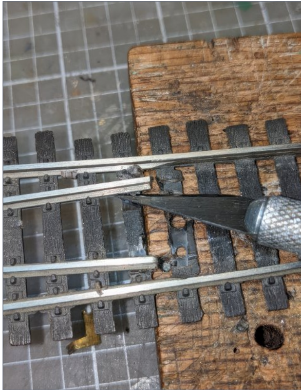
17. Use a sharp X-Acto knife to carve a pocket under the rails to make room for rail joiners.
