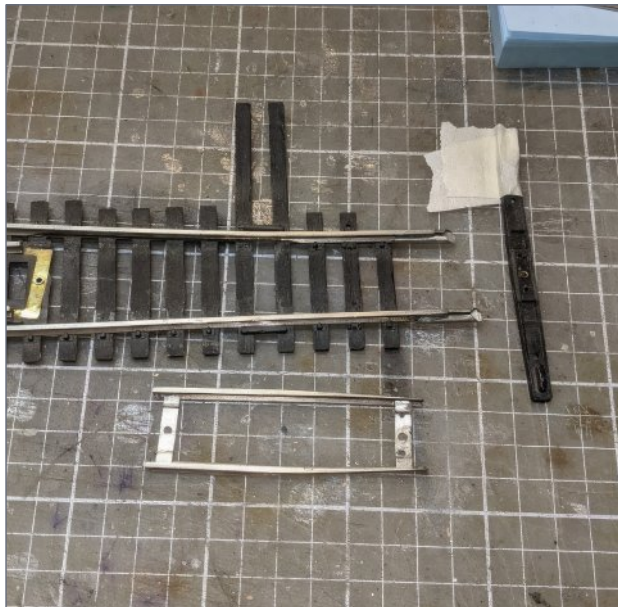
8. The turnout is separated into three pieces: the point assembly, the throw bar, and the body of the turnout.
