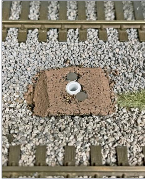
5. The magnets are in place on either side of the styrene tube.
