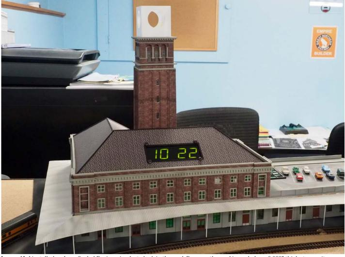
**Image 41.** I installed an Iowa Scaled Engineering fast clock in the roof. Because the roof is made from 0.080" thick styrene it needed no bracing. The roof also provides bracing for the 2nd floors walls. The 2nd stage of the clock tower is now installed and I've started the 3rd level. The 1st floors awning is complete, I cut that by hand.
