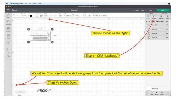
Image 04. A screen shot of Cricut Design Space. As the SVG File is up-loaded everything becomes grouped into one object. Note the overall length is 0.645 inches which is too short. The objects will also be a long way from the upper left corner of the Design Space.
