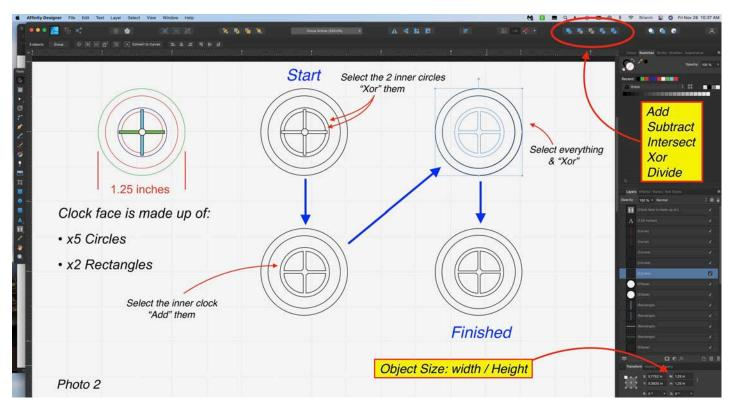
**Image 02.** The KSS clock face as drawn in Affinity Designer. From left to right: - the clock face is drawn to scale as a series of circles (in different colors to make it easier to see) and rectangles. For some reason when I Xor'd the inner part of the clock it disappeared as the stroke thickness becomes zero. I
