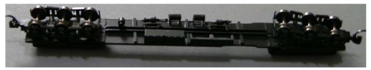
The underbody of the Wheels of Time kit has a low centerbeam with cross members typical of "Harriman" style cars, but the holes for truck bolster pins are spaced for the offcenter design used on old Micro-Trains 6-wheel trucks with 33" wheels, which are not prototypical for these T&NO cars. The battery box is inset too far from the inner edge of the car's side as well. Rather than making corrections to the resin-cast floor, I opted to construct a replacement floor using the bolster ends
