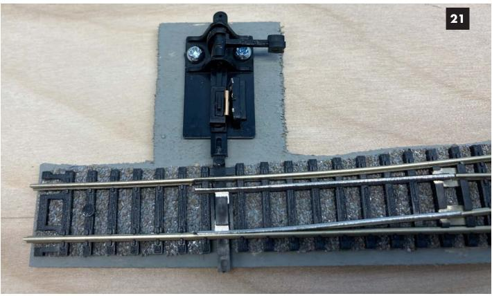
**Image 21.** Everything is in place and the unit is ready for wiring. Notice how the copper contact is only touching two of the three wiring connectors. The center post is for the frog and the two outer ones feed the correct polarity when the copper contact strip moves into place.
