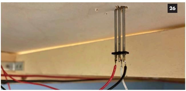
**Image 26.** The outer wires are to grab power from the bus, and they align with the outer wiring connectors as they are lined up with the inner and outer rails of the trackwork.
