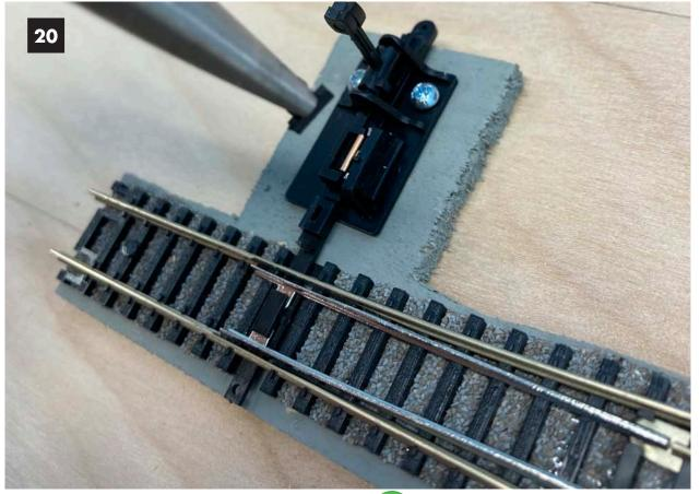
Image 20. The copper contact strip is held in place by a plastic cap, the flat side goes against the copper contact strip.
