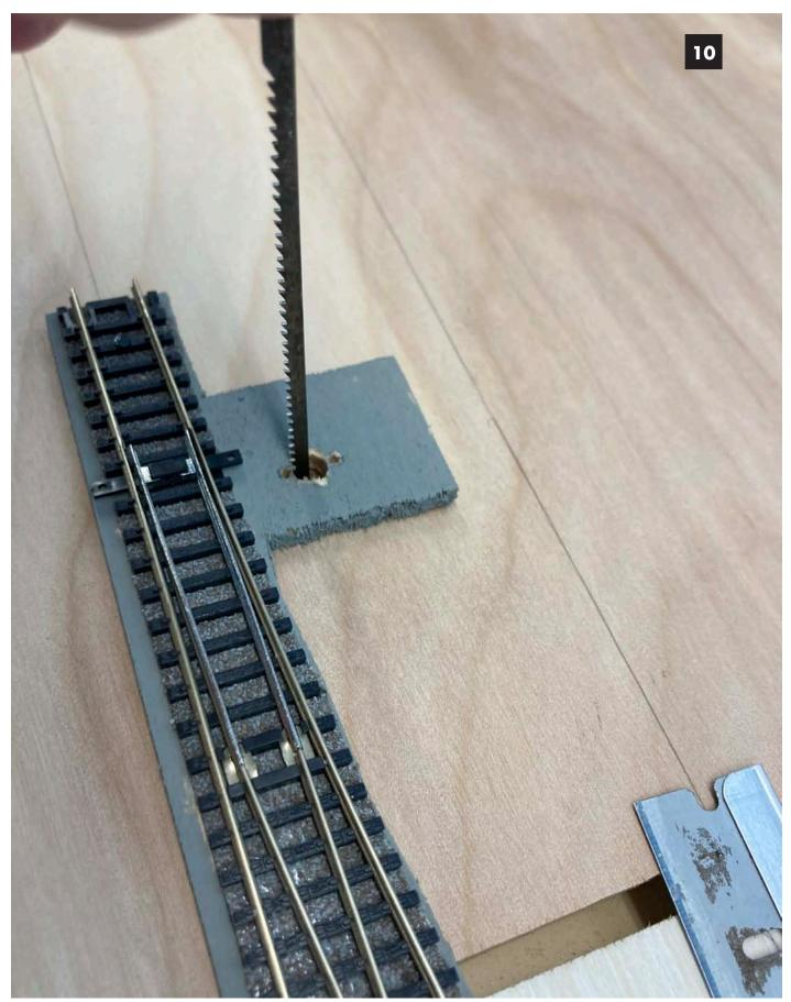
**Image 10.** I use a naked coping saw blade to carefully enlarge the hole into a slot for the wiring connector. This is truly easier than it looks and sounds. My benchwork here is ½" Baltic birch plywood, if it were a thicker base, it would be a little more tedious.
