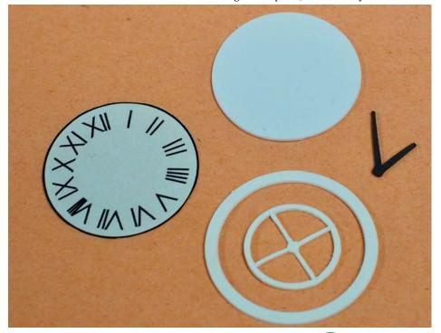
**Image 42.** The clock face was printed on paper while the hands and rings were cut with the Cricut Maker. The Maker is exceptionally good at cutting circle components out of styrene.
