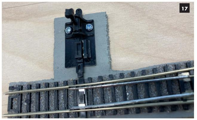
Image 17. After the wiring connector is snapped in place, the tops of the three metal strips are visible.
