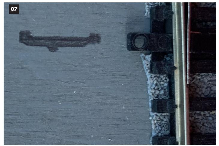
**Image 07.** This shows the outline made of the slot in the base of the ground throw. This area must be removed all the way through the turnout block and the benchwork in order to install the wiring connector.
