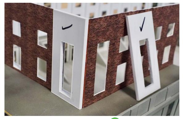
Image 25. All the corners of the KSS project outward from the base walls, I was able to simulate this with 0.080" thick pieces of Evergreen styrene, which I scored on the Cricut Maker. I snapped the walls along the outer cut lines. I used a #18 X-Acto chisel blade to finish the cut for the inner window. I placed the #18 blade into the score line and then rocked the blade back and forth while applying pressure to finish cutting through the styrene. This takes time, but it worked.
