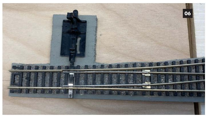
**Image 06.** The ground throw is placed in position with the switch points centered and the throw in a vertical position to line things up.
