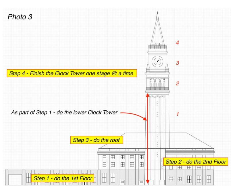
**Image 03.** One my early illustrator drawings of King Street Station with my basic plan of how I would break down the construction into sections of work.
