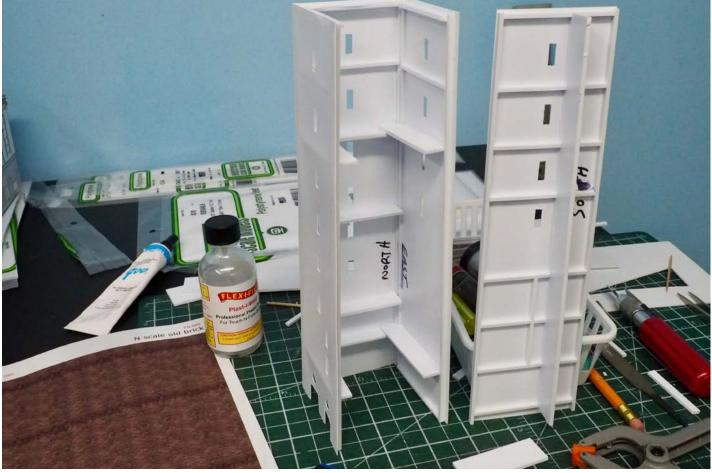
**Image 14.** This is the lower section of the clock tower. I braced this with the #166 strips plus scraps of 0.080" styrene. I added more bracing than this photos shows, but you get the idea. I also left the south wall unglued as eventually I would need to add window glazing.
