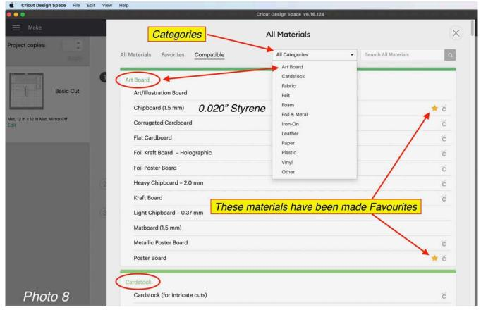
**Image 08.** Pick the type of material that you're going to cut. By marking you're commonly used materials as a Favorite, you will see them as a clickable selection (Star) and reducing the need to scroll through a long list, as shown in the photo.
