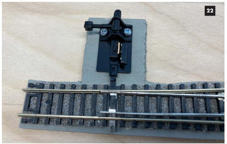
Image 22. The contact strip moves with the ground throw mechanism to correctly line up the correct polarity.
