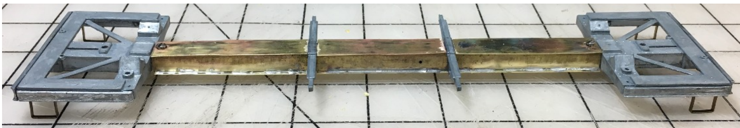
Above: All 6 pieces soldered and the new holes drilled for the screw to hold the end sills.
