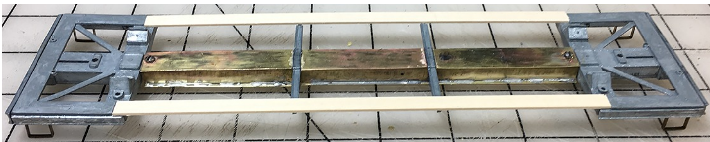
Above: All 6 pieces soldered and the new holes drilled for the screw to hold the end sills.
