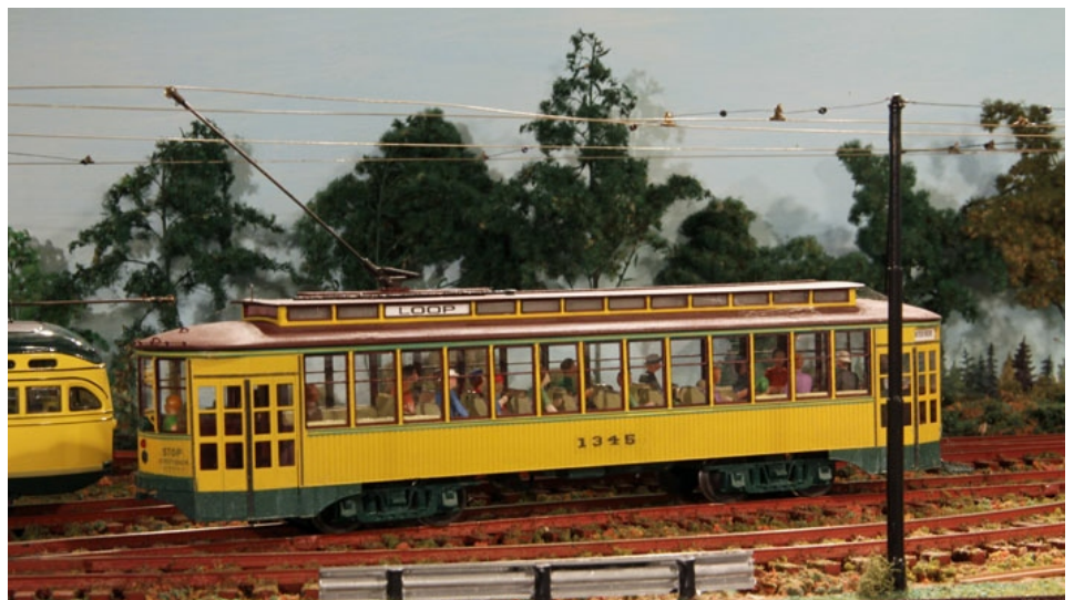
Number 1345 is one of the home built Twin City Line cars. This model is a limited production kit produced by Dave Waddington, These were etched brass kits. The basic body was built by Dick Stoner and Forrest finished it.
