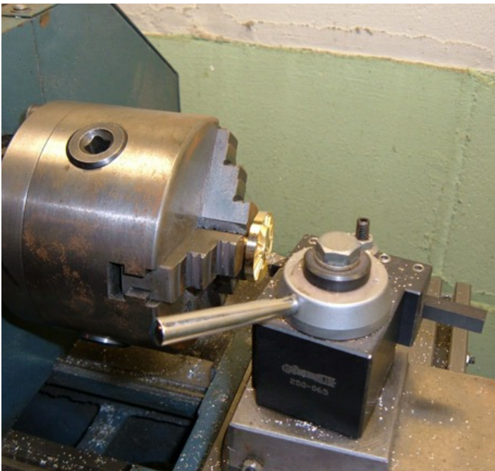
These two photos show turning the outside diameter of the rim and facing the hub. When measuring, use a micrometer. A caliper will not be accurate enough.
