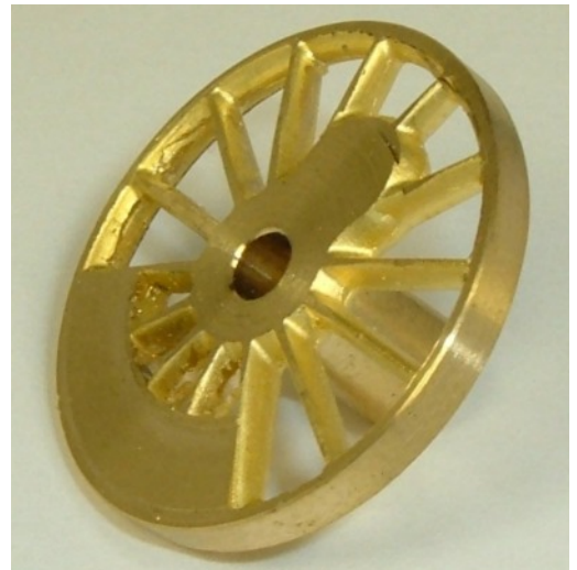
The finished driver center ready to cut the boss off of the back.
