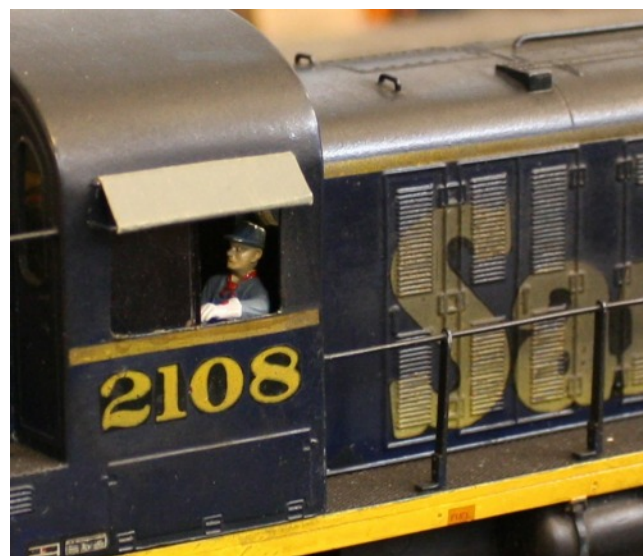
In this close up view of Jim DeBruin's RSD-4/5, you can see the raised door outlines of the early etching. Also, you can see that the outline of the window just ahead of the fireman's hand is irregular. This was because the window had to be cut out by the modeler, and it was difficult to keep the line straight.
