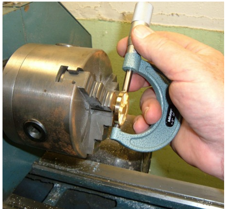
These two photos show turning the outside diameter of the rim and facing the hub. When measuring, use a micrometer. A caliper will not be accurate enough.
