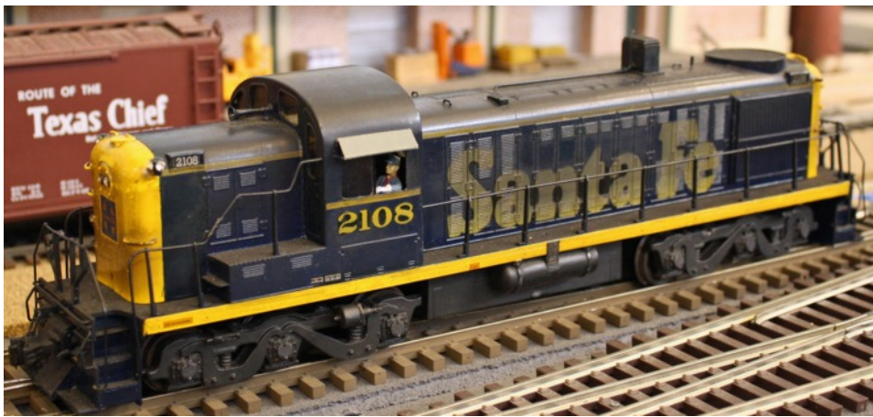
Jim DeBruin owns this early Kemtron RSD-4/5 model, and sent me the photo. Note that on this model the truck side frames are a one piece casting. These are Central Locomotive Works trucks. The Kemtron trucks were sprung and equalized.
