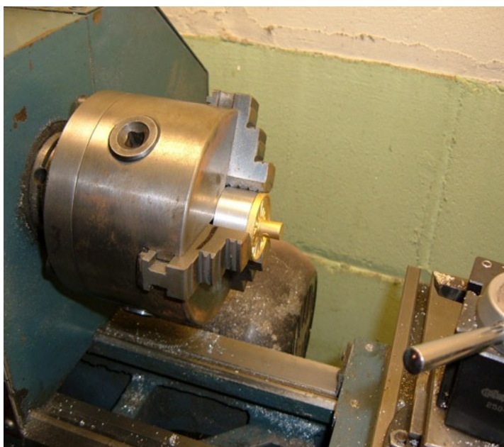
These two photos show the spacer that I made in place in the chuck. On the right is the machined boss, which is now perpendicular to the face of the rim.
