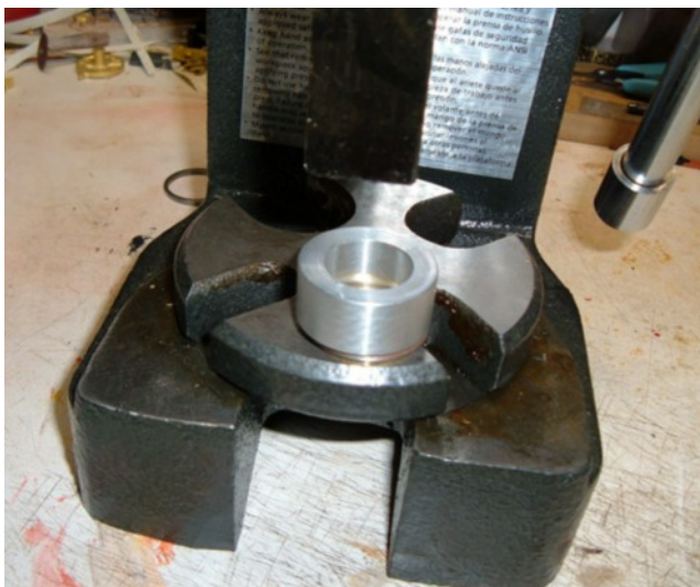
The final operation is to press the tire on the rim.
