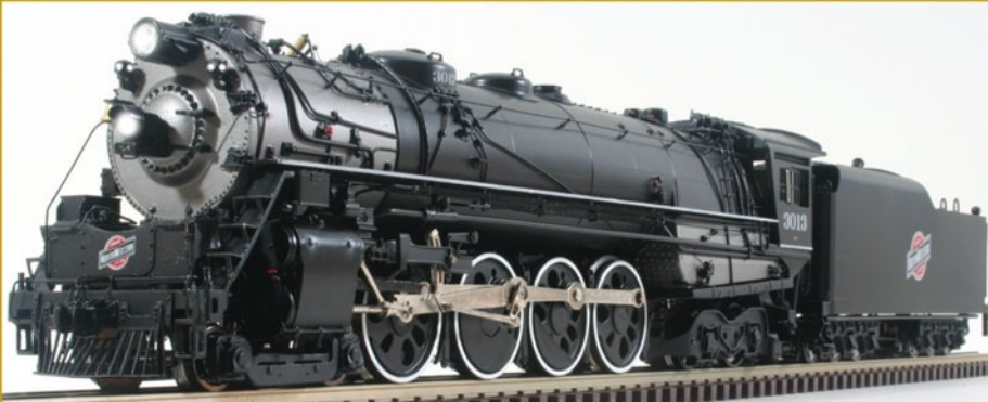
Chicago & North Western H-1 4-8-4 In 1929 C&NW received 35 very large 4-8-4's from the Baldwin Locomotive Works. They were some of the largest 4-8-4's ever. In the late 1940s, the entire fleet underwent a rebuild to include lightweight rods, boxpok drivers and roller bearings on all axles. These were reclassified as H-1. New Railsounds ("AWESOME") In Stock Now!!!, Only 60 units made. Pittman Powered, Sprung Drivers, Lighting
