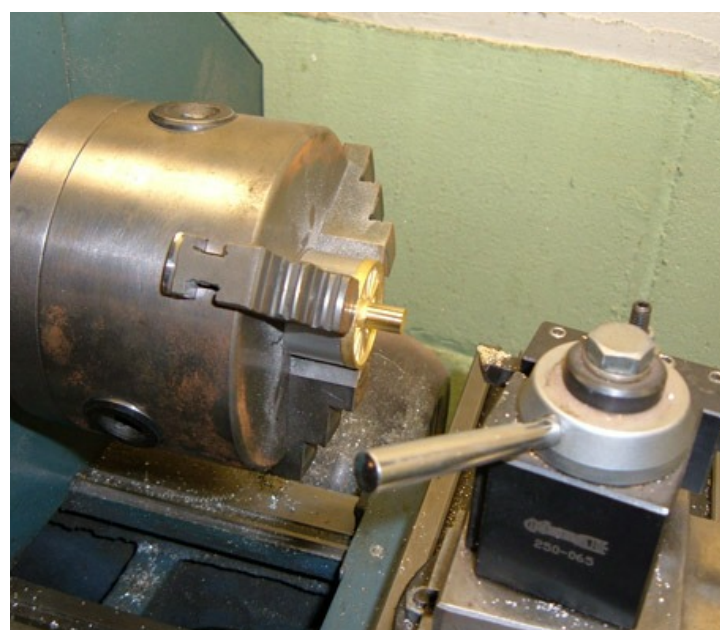
These two photos show the spacer that I made in place in the chuck. On the right is the machined boss, which is now perpendicular to the face of the rim.
