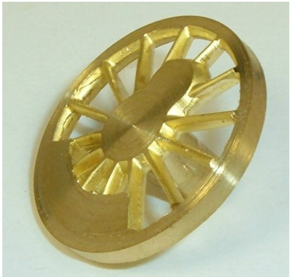
This was my first attempt at machining a driver. Note that the spokes in the foreground are machined through at the rim and the ones in the background are not. This is NOT what we want.
