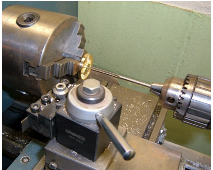
The last operation is to ream the hole to size.
