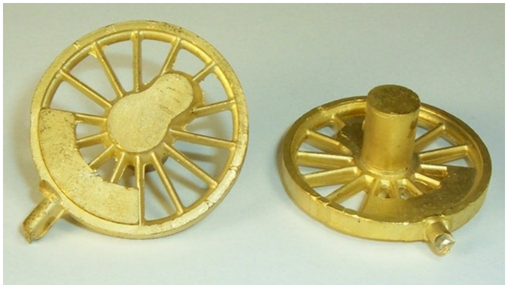
These castings are typical of what you will get when you buy driver centers.
