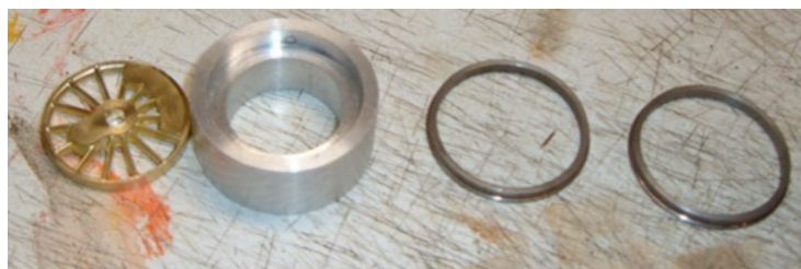
The finished driver center, tires, and press tool
