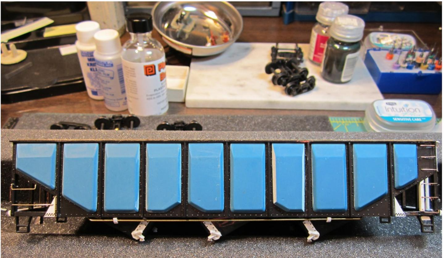
*Above: A side view of the model nearing completion of the detail. The resin panel sides have been added, as well as, additional hopper details including latches from SHS. I added the gussets at the ends as support for the slope sheet as shown on the prototype photo and also used some Archer rivet detail.*
