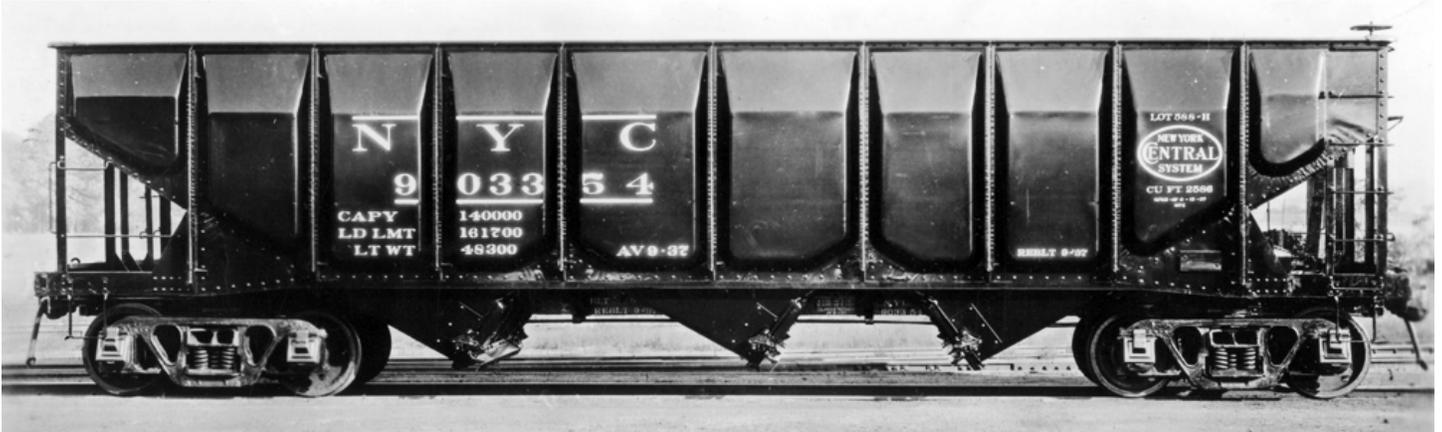
*Above: NYC 903354 is one of the 70-ton panel side hoppers designated Lot 588-H following a major rebuilding in 1937 where the panel sides and the center saw-tooth hopper outlet were added. The work was done at "AV" in September 1937. That would be the New York Central's Avis, PA shops. This photo is courtesy of the New York Central System Historical Society.*
