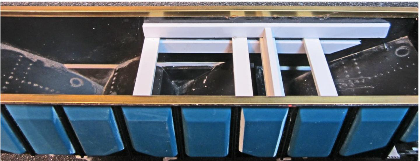
*Above: Another view of the 0.080" x 0.375" styrene reinforcement as well as a bit of the styrene shims used to reattach the center hopper outlet bay.*
