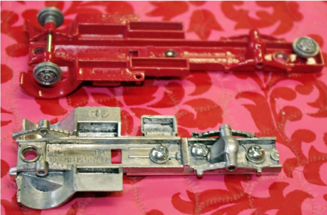
*This photo shows a stock chassis at the top, and one Roy modified at the bottom. He cut a stock chassis and screwed it back together using a piece of aluminum for a splice plate. Roy said sometimes you need to cut off fuel tanks to make them smaller, but it is not hard to get a chassis of the right length for what you want to do.*
