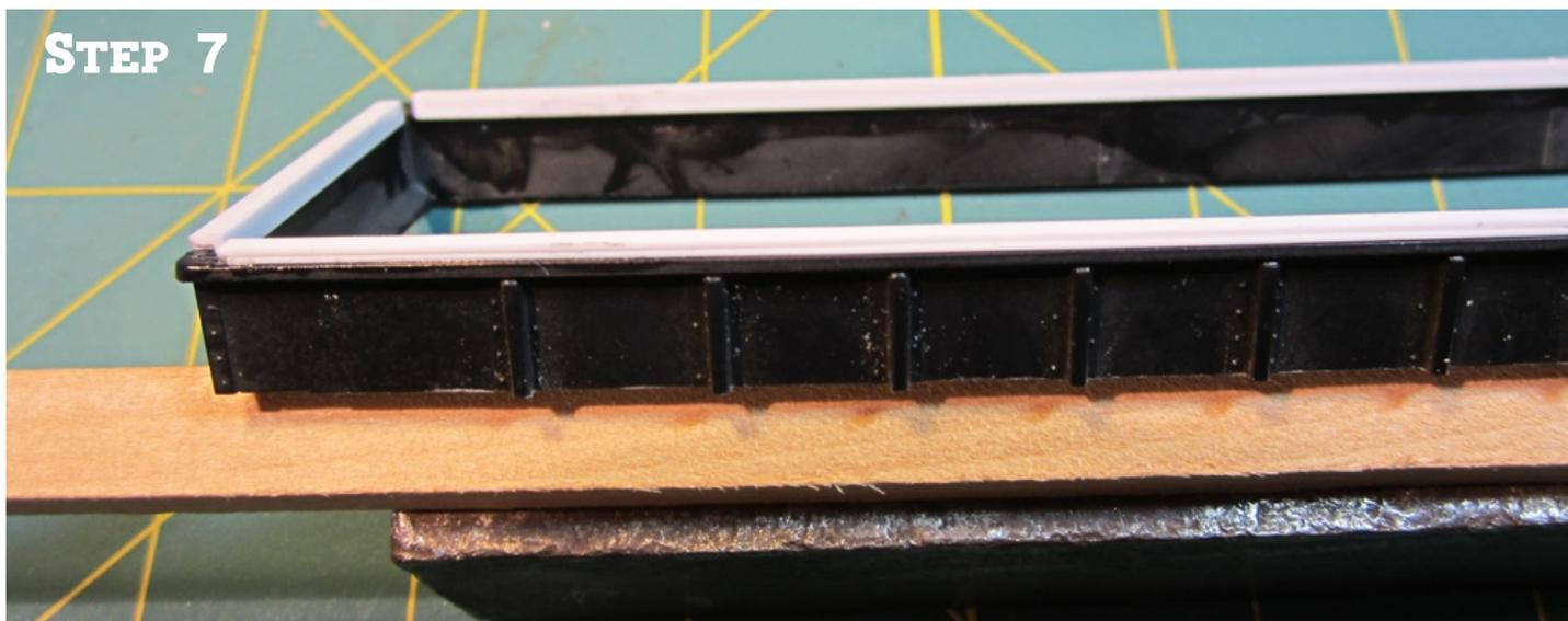
Step 7: The finished cut extension piece should have a straight cut with very little flash. Only a minimal amount of filing clean-up will be required. I glued a strip of 0.015 styrene directly to the piece and then topped that with 1/16<sup>th</sup> x 1/16<sup>th</sup> styrene angle to add a bit more height to the model and strength to the extension piece.
