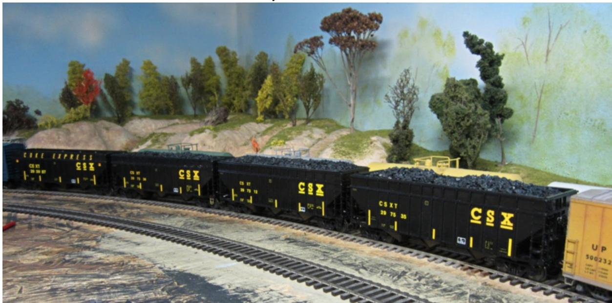
*Three photos (above and next page) of a completed string of cars on Chuck West's Des Plaines Valley layout. The "Coke Express" car runs as an empty, the others carry simulated coke loads. The material is coarse coal from Arizona Rock & Mineral. After gluing the pile together like you would ballast, I hit it with a light spray of Scalecoat MOW gray. That gives the load a slightly lighter, grayish color, an effect more closely imitating the appearance of coke.*
