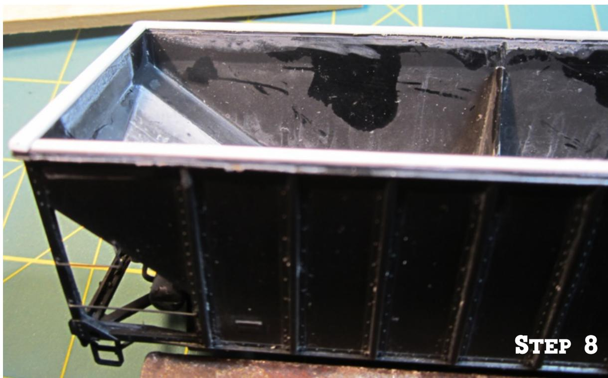
Step 8: I also added a strip of styrene to the top of the lower portion of the hopper. This is not entirely necessary, but I found the styrene gives a better surface for gluing when it is time to attach the extension.
