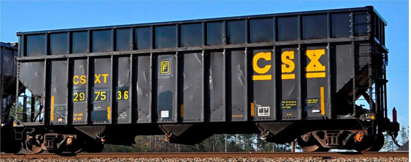
*A big note of thanks to S Scale modeler, Pete Silcox, who provided this photo of a CSXT extended height coke hopper. The extended portion has been built on top of an existing hopper. While the existing car is likely not one of original Pennsy or C&O H39 hoppers, it does have 13 ribs, exactly the same as the S Scale H39 model. This photo was taken by Pete's friend and fellow CSXT employee, John Jones, on December 14, 2011 in Waterloo, South Carolina.*
