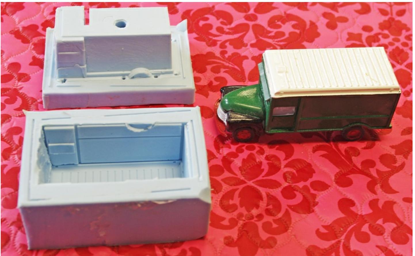
*The Railway Express company had very distinctive trucks much like United Parcel Service does today. Roy is developing a kit of one. In the top photo, you can see a finished truck and a raw casting of the box. In the bottom photo, you can see how the two part mold looks like that Roy casts the box body in. These are complicated molds to make and to fill with resin.*
