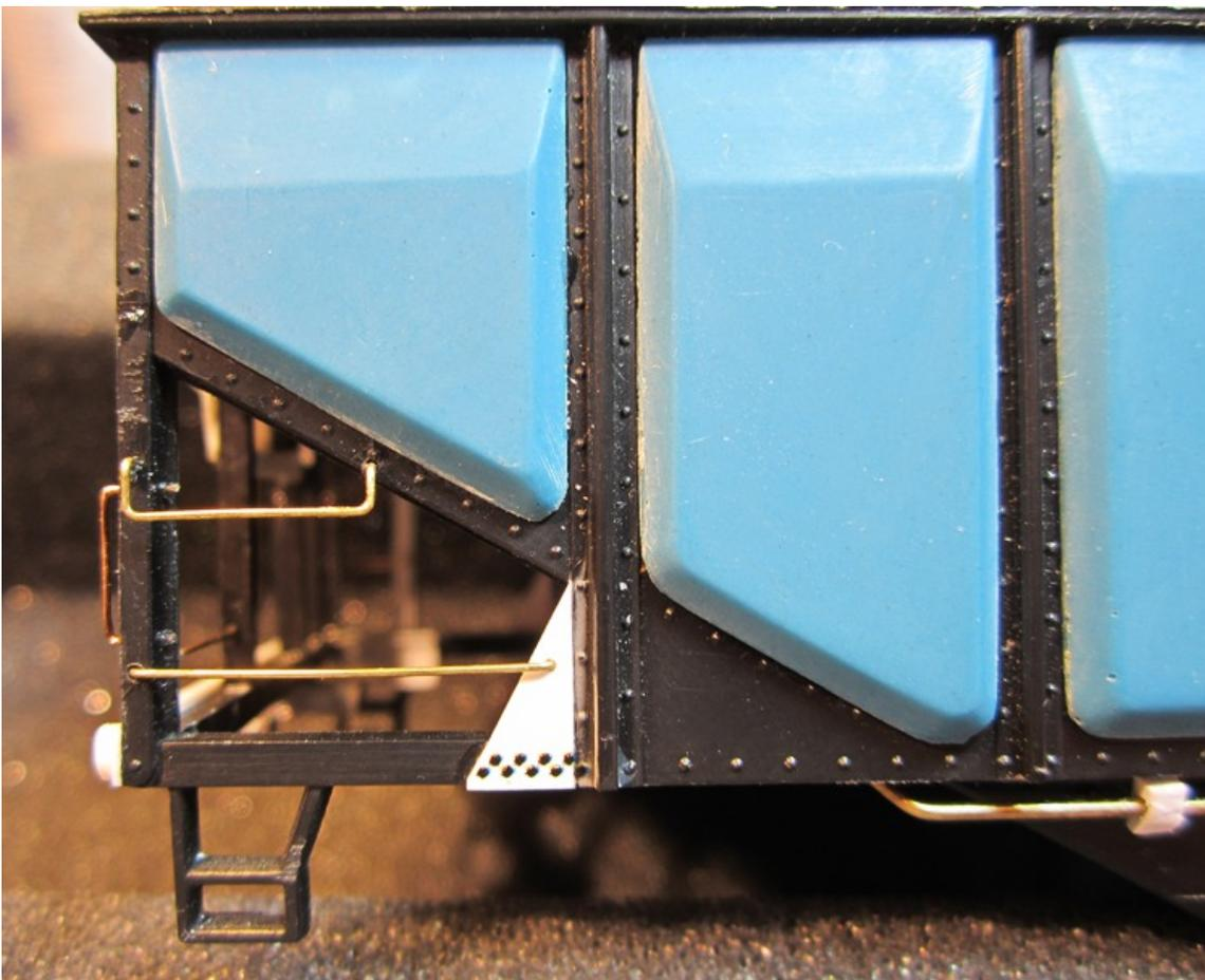
*Left: This photo is a close up of added detail including the slope sheet support gussets, some Archer rivets, and fabricated grab irons.*
