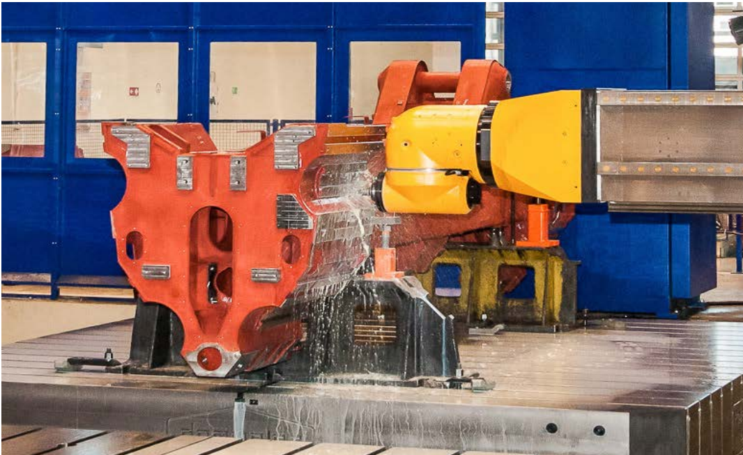
Figure 34: Tos Varnsdorf (Czechia) machine tool 52 milling an erector
