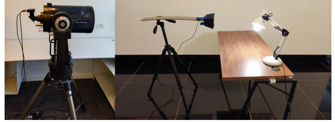
Figure 17: Experimental setup: An electro-optical sensor is mounted to a telescope (left picture) that is directed at a desk lamp light bulb (placed 50 cm from the speakers) from 35 meters away (right picture).
