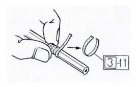
Apply a drop of light machine oil to 3-11 Teflon Strip as instructed with the sign in the illustration and install 3-12 Eccentric Strap and 3-13 Eccentric Strap around the bearing of 2-21 2<sup>nd</sup> Coupled Driver using M1.7-4 screws. Attach 3-14 Axle Driven Pump Rod to 3-13 Eccentric
