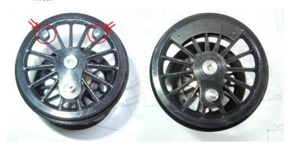
2. Attach 2-5 Counter Balance Outside for 3<sup>rd</sup> Driver to the outside of 2-4 Main Coupled Driving Wheels and attach 2-6 Counter Balance Inside for 3<sup>rd</sup> Driver to inside of 2-4 Main Coupled Driving Wheels fastening M1.4-5 screws as shown with
