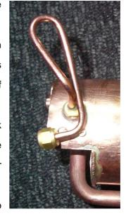
4 kg/cm², carefully check water leakage from joints and fastenings, marking the leakage area if any. After you finish checking all the leaky area, drain the water from the inner boiler to remove the leaky fitting and repack the threads with packing compound. Repeat the same sequence until you verify that no leak is present.
