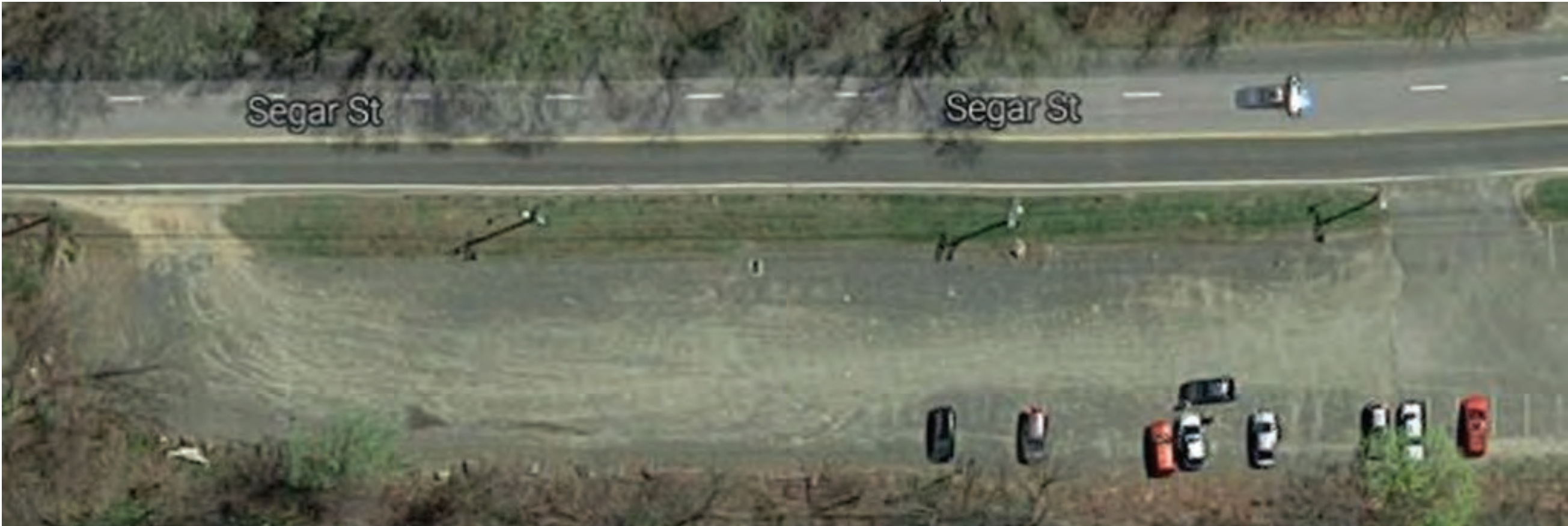
The fence bordering the lot near a small stream is in disrepair. The angled posts on the fence may be evidence of soil creep on the slope down to the stream.
