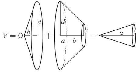
$$\begin{aligned} V &= \frac{\pi}{3}bd^2 + \frac{\pi}{3}(a-b)(c^2 + cd + d^2) - \frac{\pi}{3}ac^2 \\ &= \frac{\pi}{3}(ad - bc)(c + d). \end{aligned}$$
