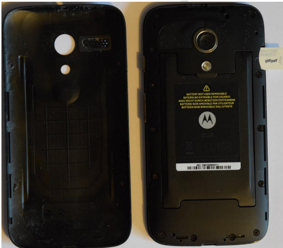
Mobile handset with cover removed - note the slot for the SIM card in the top-right and that the battery is accessible but not designated as user-removable
