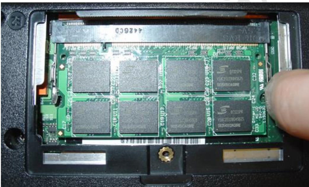
Open the panel to access the RAM module(s) then flip the catch to pop the card up
