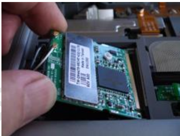
Adding a Mini PCI wireless adapter - note the wires for the antenna on the left
