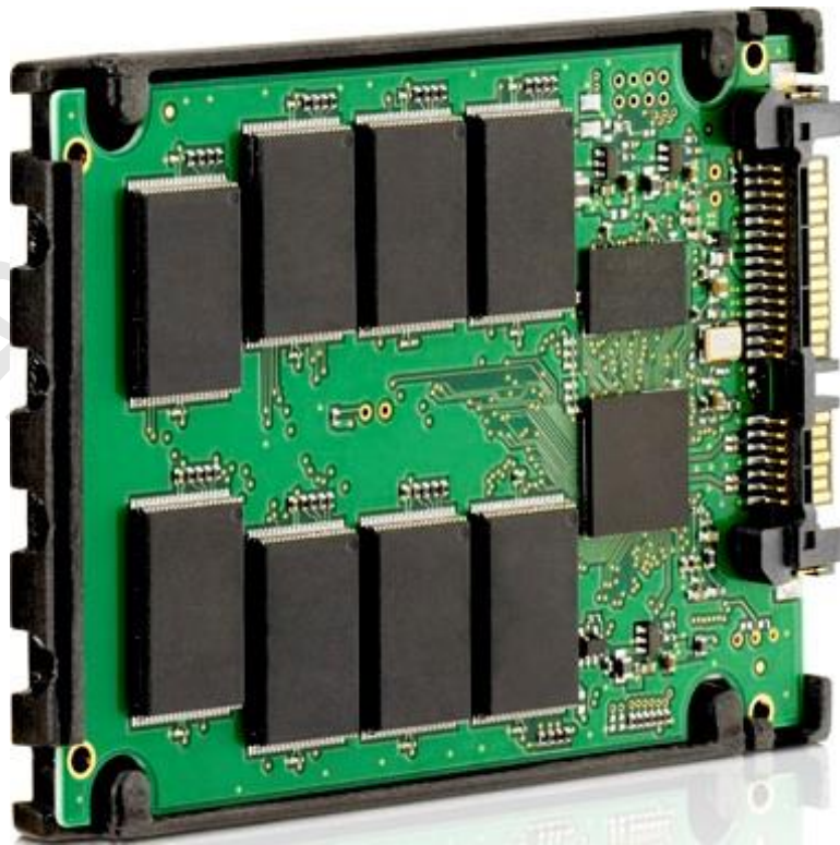
HP SSD with SATA interface (© Hewlett-Packard Development Company)
