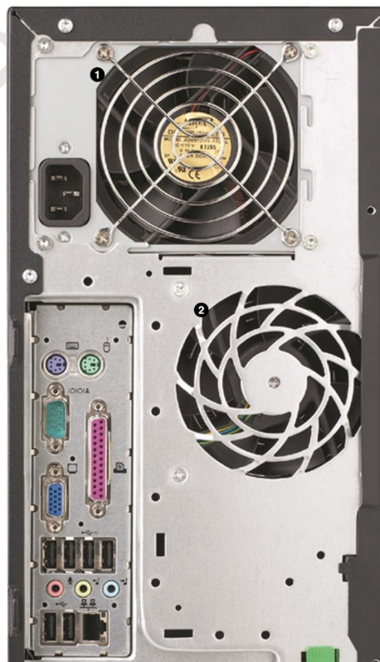
PSU (1) and chassis (2) fans on an HP Compaq PC (© Hewlett-Packard Development Company)
