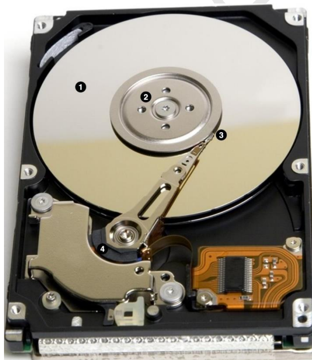
HDD with drive circuitry and casing removed showing 1) Platters; 2) Spindle; 3) Read/write heads; 4) Actuator
