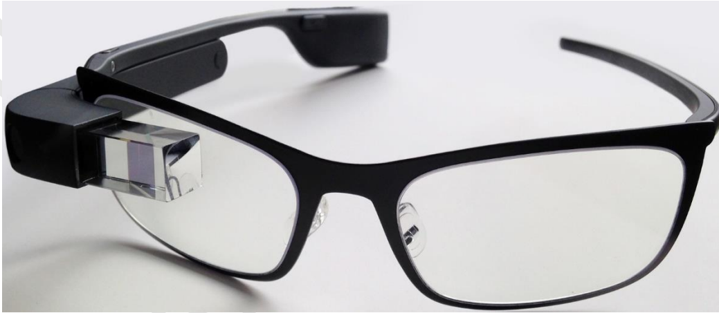
Google Glass featuring camera and OHMD (Image courtesy Mikepanhu / Wikimedia Commons CC-SA-3.0)
