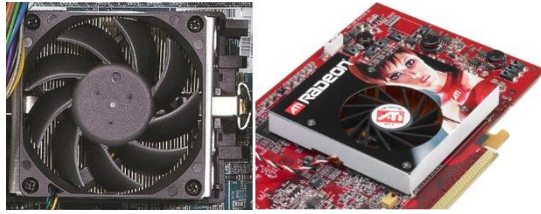
Fan assembly on a CPU (left) and ATI Radeon graphics processor (right)
