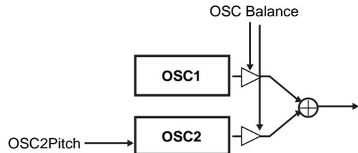
WAVE ..... Osc1(Saw, Squ, Tri, Sin) + Osc2(Saw, Squ, Tri, Sin, Ns[=Noise])
