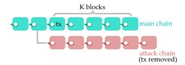
Figure 14.1: The adversary aims to undo transaction tx by mining a longer fork than the main chain. If the adversary has only minority of the mining power, statistically speaking, it is extremely unlikely that the adversary can win the race against the main chain. Let K be how deep tx is embedded in the main chain: as K increases, our confidence in tx's finality increases very sharply.
