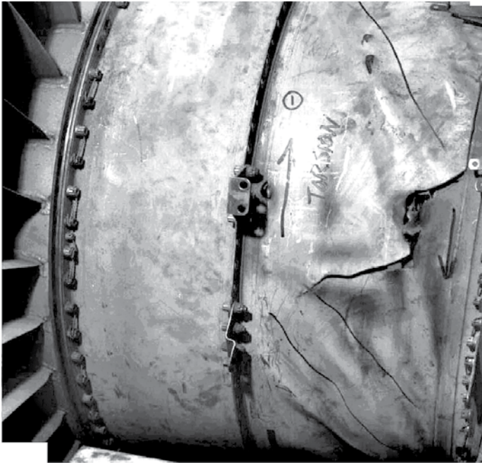
Figure 2. Torsion buckling in an engine case.
