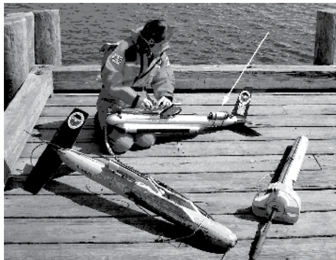
Figure 3. The heart of imaging sonars are transducers mounted on a hydrodynamically streamlined structure often called a “towfish.” Note the relocation pinger on the aft end of the silver towfish (arrow). This is very similar to those attached to DFDRs and CVRs. In the event the tow cable is severed by fishbite or an obstruction, the pinger transmits a signal allowing it to be located and recovered.
