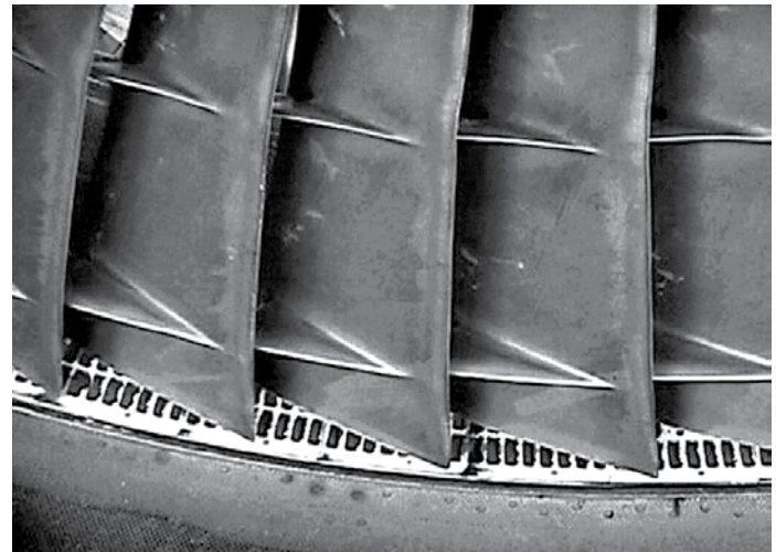
Figure 7. Fan blade tips seized into fan case.
