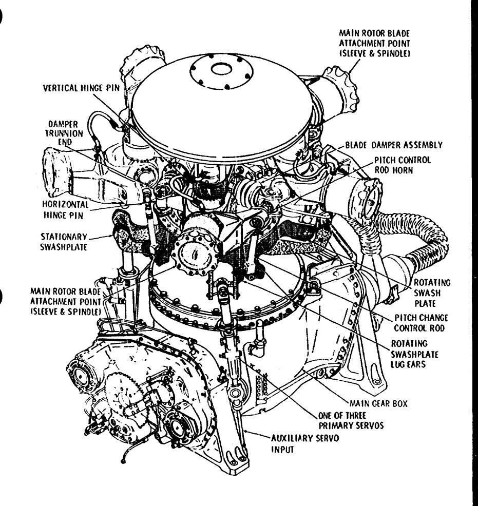
Attachment 1. Explanatory Diagram of Main Rotor Head
