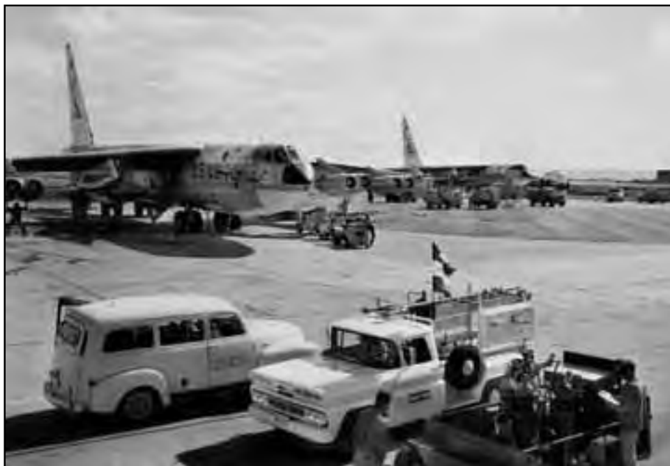
On 4 November 1960, the program attempted to launch two X-15 flights in a single day. Here X-15-1 is mounted on the NB-52B and X-15-2 is on the NB-52A. Rushworth was making his first flight in X-15-1, a low (48,900 feet) and slow (Mach 1.95) familiarization. The X-15-2, with Crossfield as pilot, aborted due to a failure in the No. 2 APU. (NASA photo E-6186)
