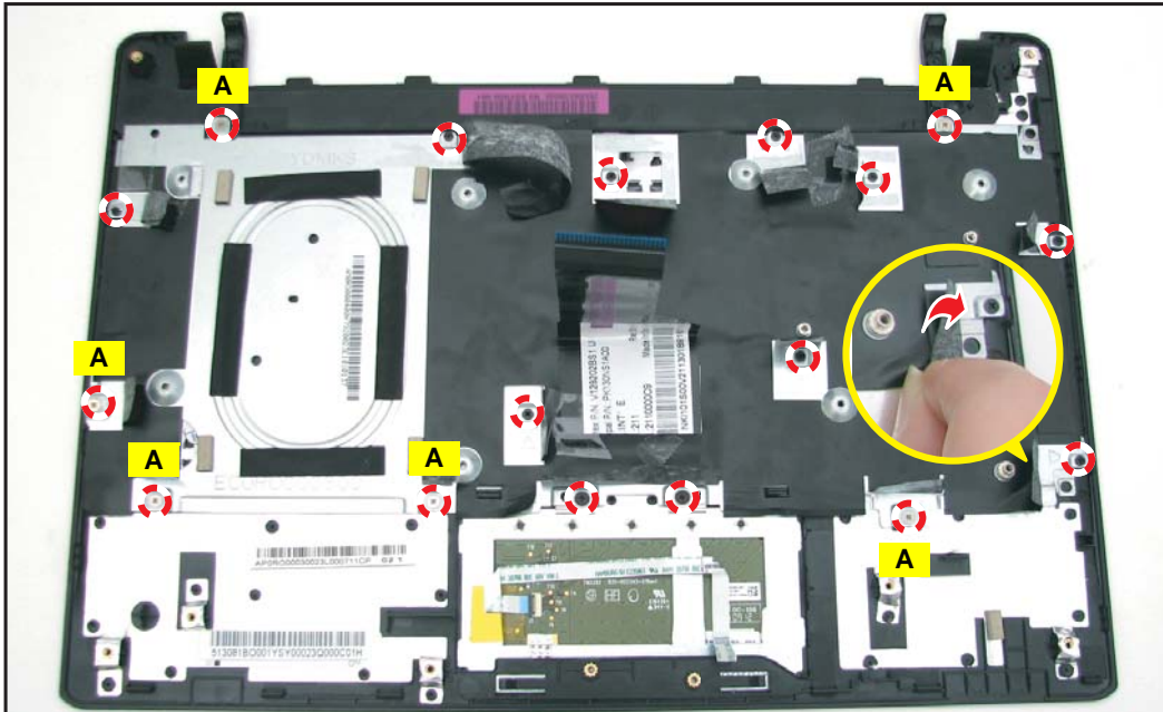
Figure 5:79. Securing the Keyboard Plastic
