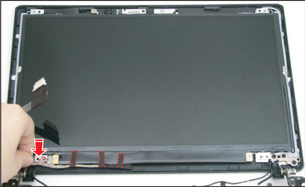
Figure 5:122. Attaching the LVDS Cable Adhesives
