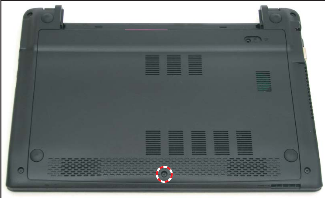
Figure 5.8. Removing the Base Door Screw
