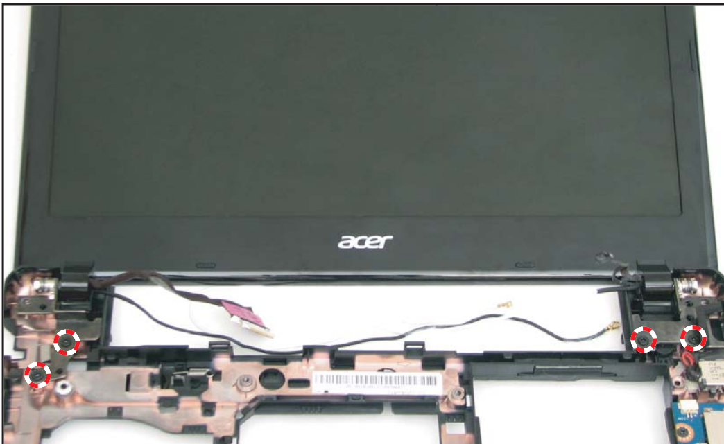
Figure 5:93. Removing the LCD Module Screws
