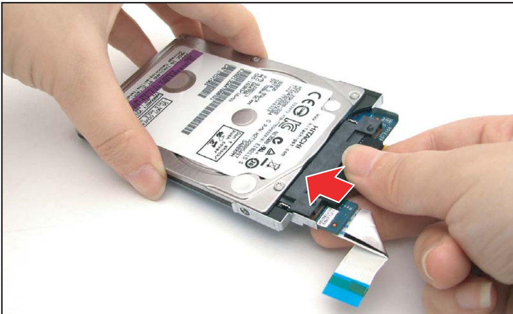
Figure 5:21. Connecting the HDD Board Connector
