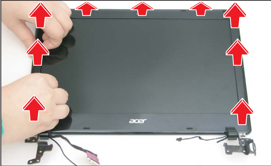
Figure 5:102. Removing the LCD Bezel (1 of 3)
