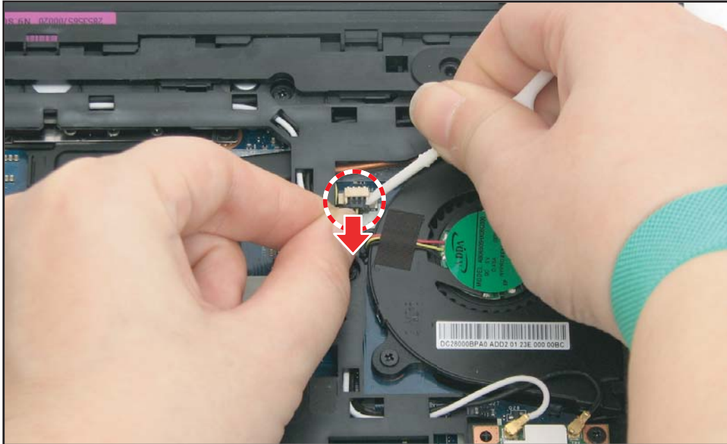
Figure 5:23. Disconnecting the Fan Cable
