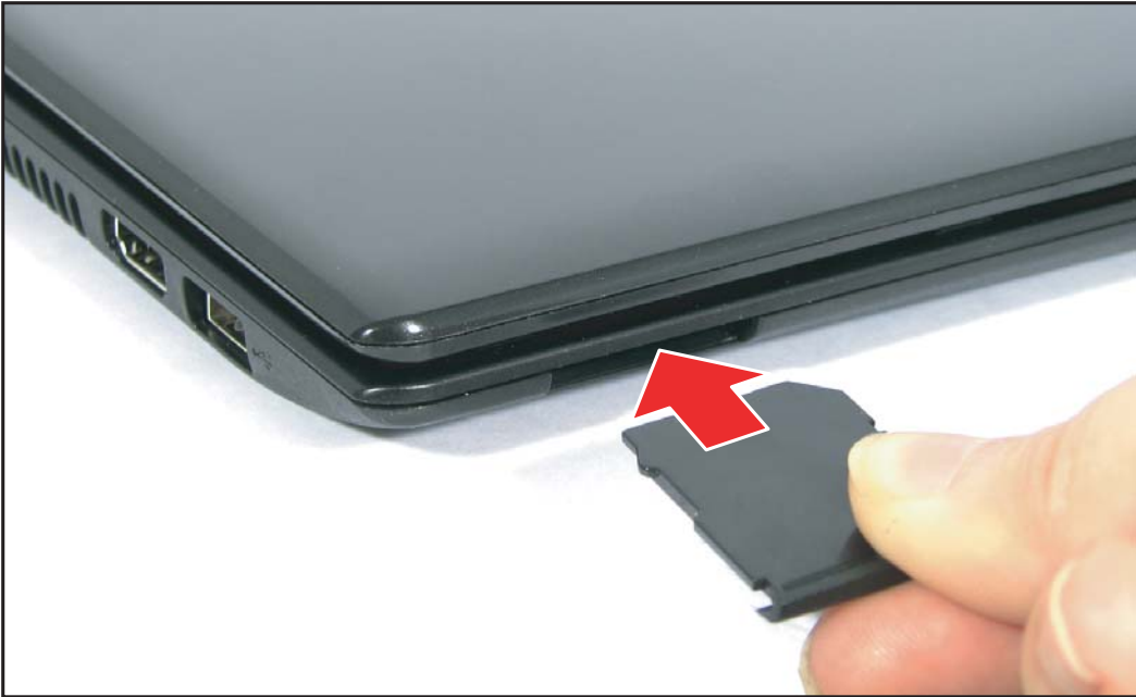
Figure 5:7. Installing the SD Card
