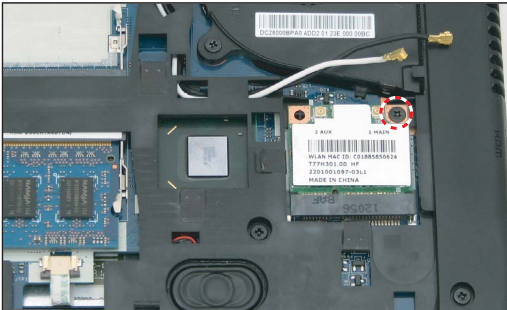
Figure 5:34. Removing the WLAN Module Screw
