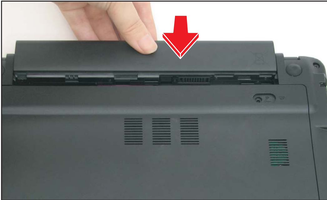
Figure 5:5. Installing the Battery Pack
