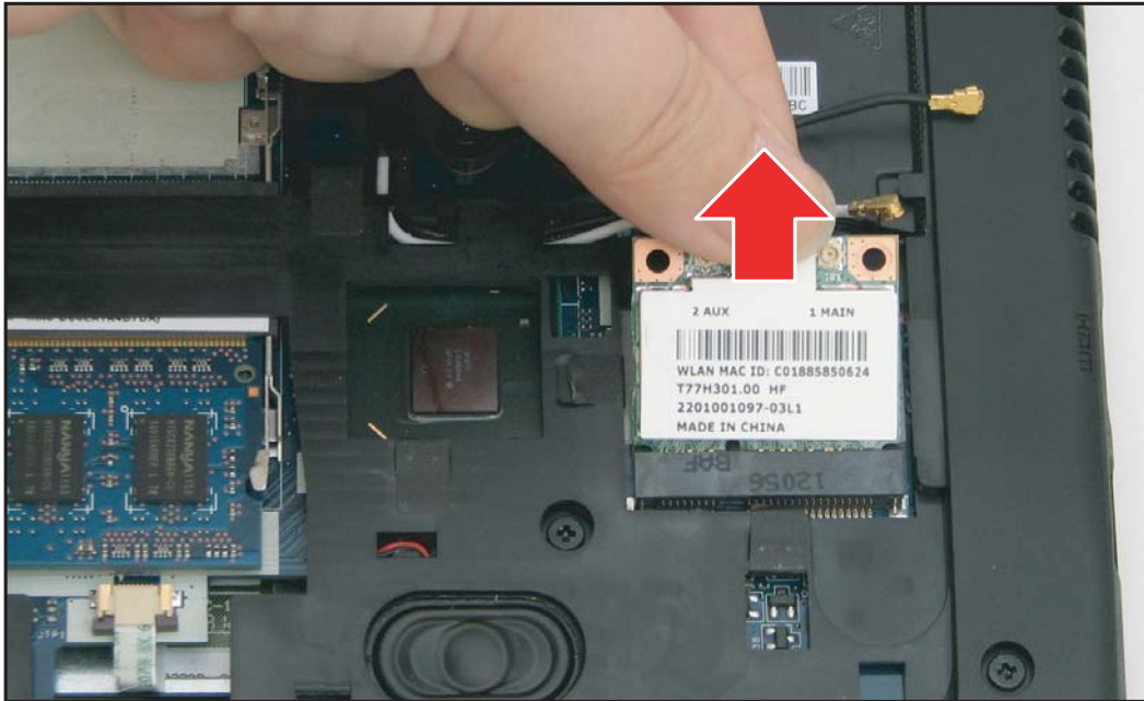
Figure 5:35. Removing the WLAN Module
