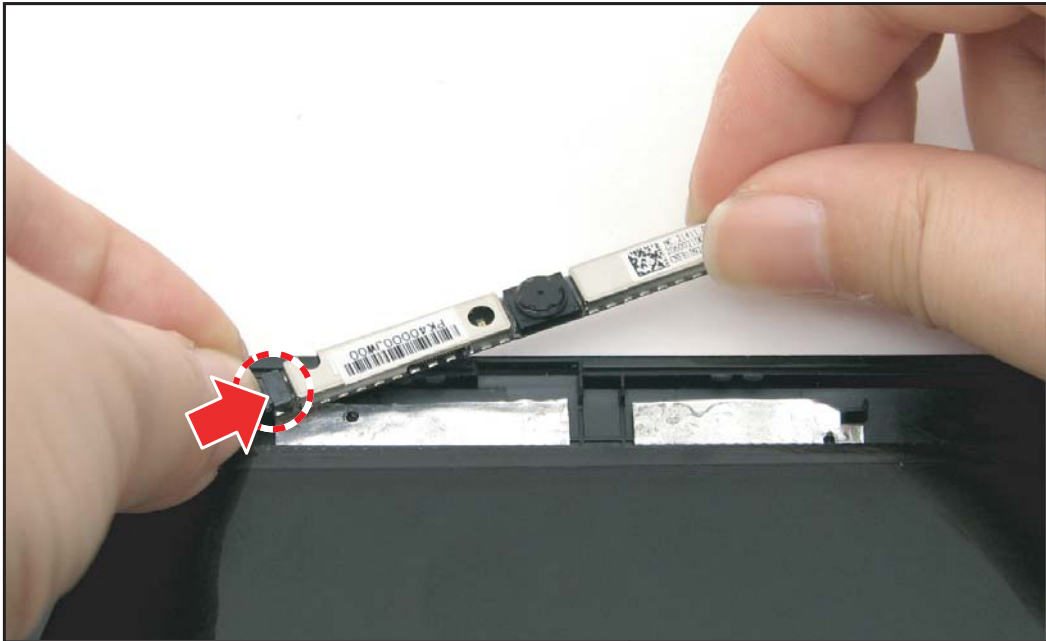
Figure 5:126. Installing the Camera Module (1 of 2)
