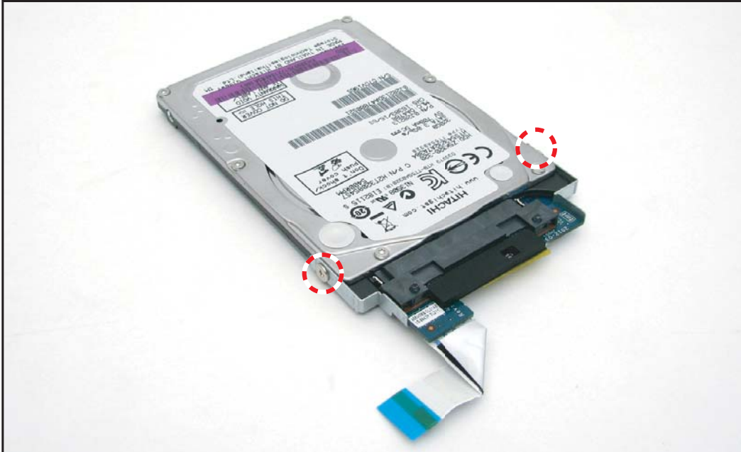
Figure 5:17. Removing the HDD Brackets
