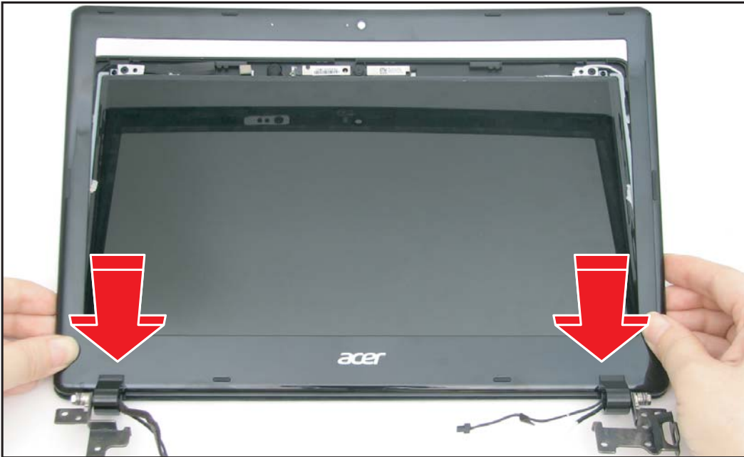
Figure 5:105. Installing the LCD Bezel (1 of 3)
