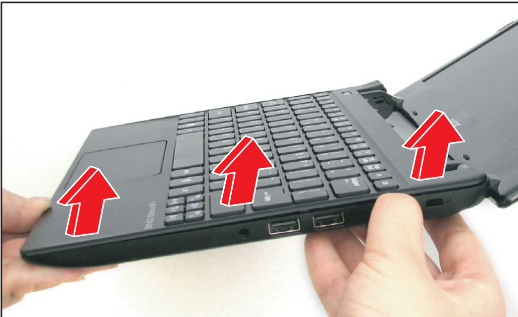
Figure 5:41. Removing the Upper Case (1 of 3)
