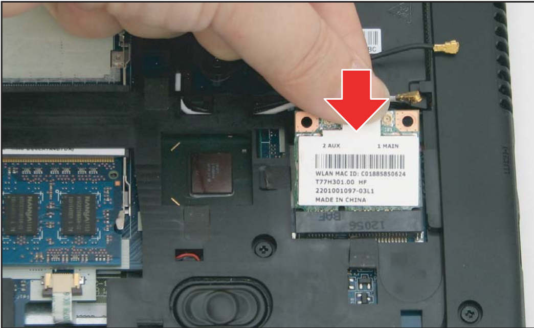
Figure 5:36. Installing the WLAN Module
