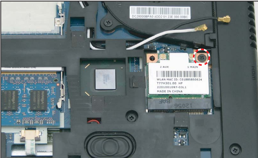
Figure 5:37. Securing the WLAN Module Screw
