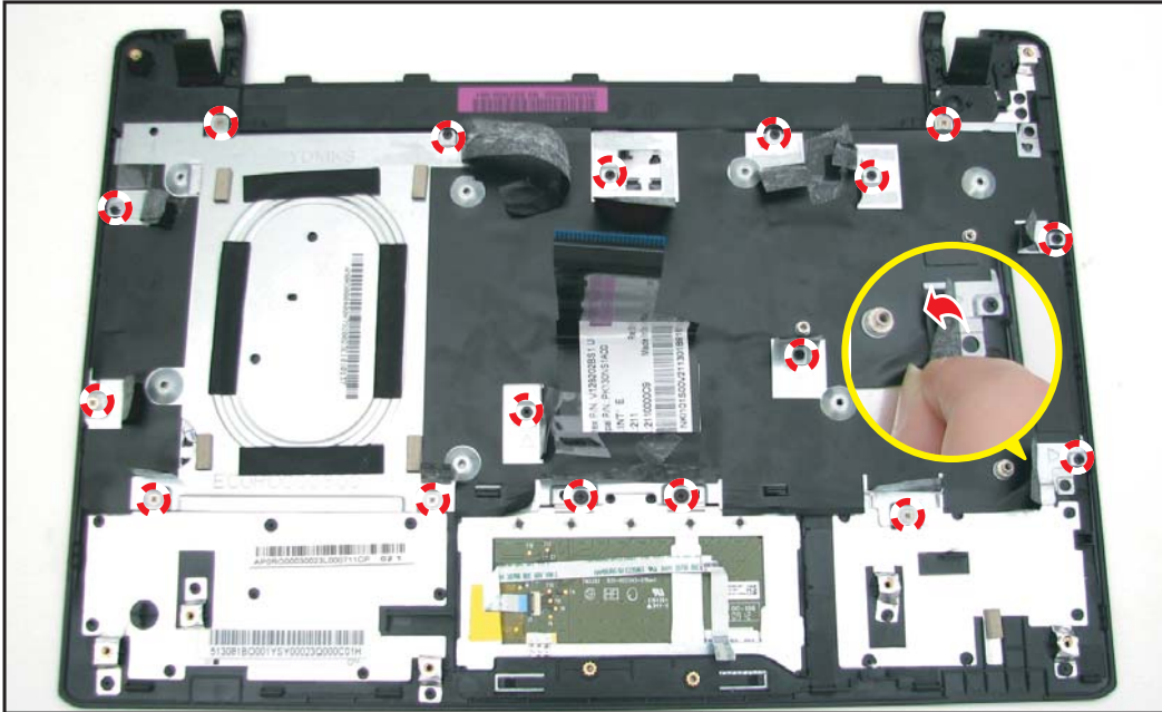
Figure 5:74. Removing the Keyboard Screws
