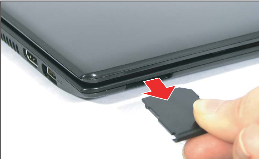
Figure 5:6. Removing the Dummy Card
