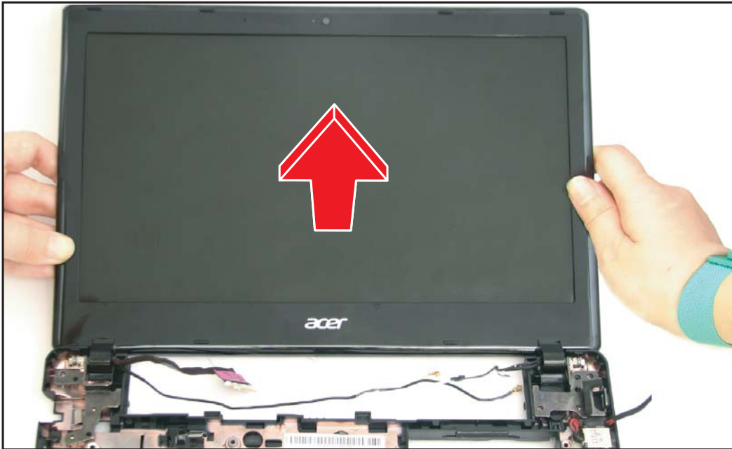
Figure 5:94. Removing the LCD Module
