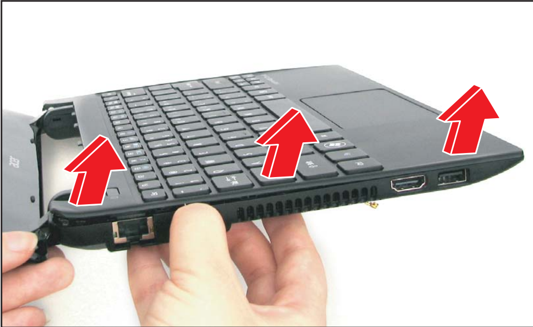
Figure 5:42. Removing the Upper Case (2 of 3)
