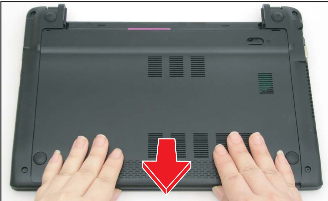
Figure 5.9. Removing the Base Door
