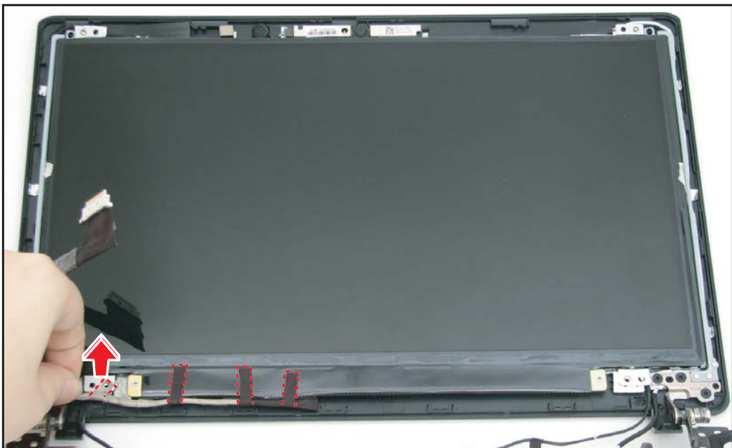
Figure 5:109. Removing the LVDS Cable Adhesives
