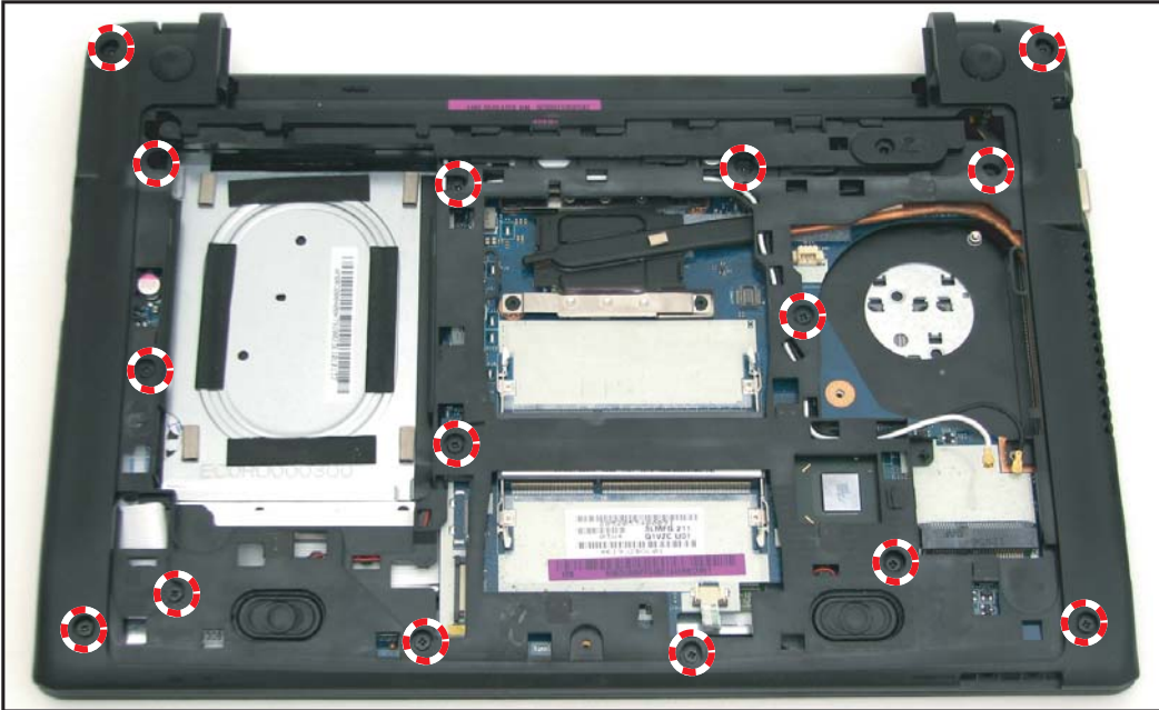
Figure 5:40. Removing the Upper and Lower Case Screws
