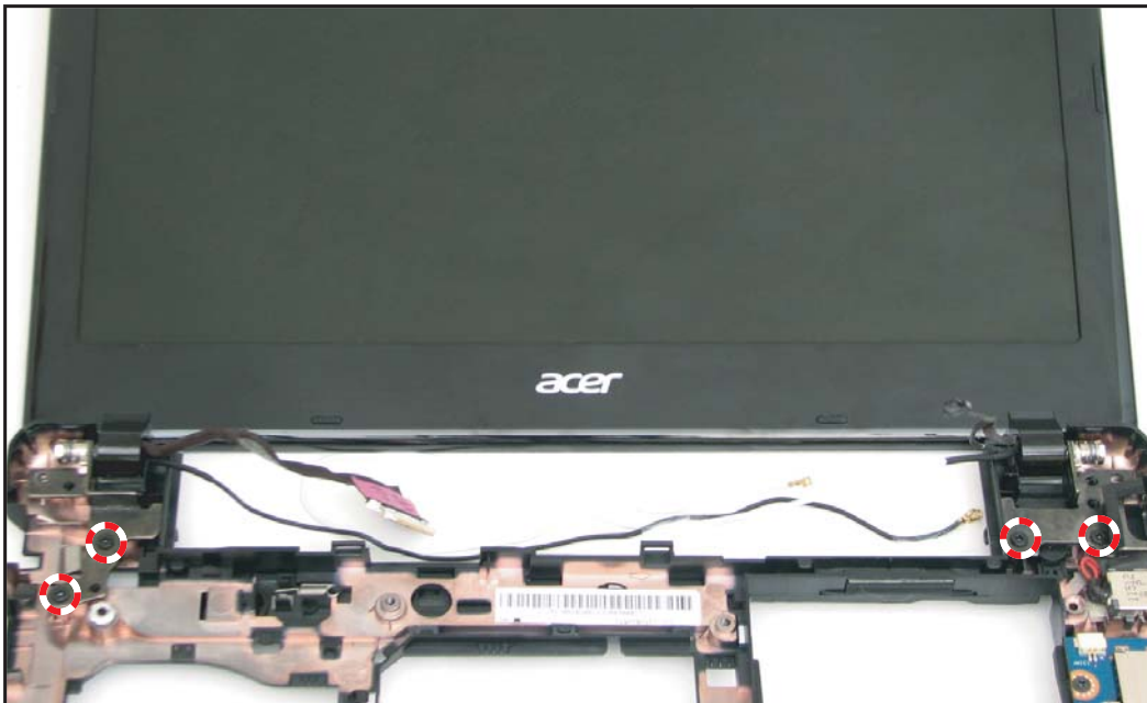
Figure 5:96. Securing the LCD Module Screws
