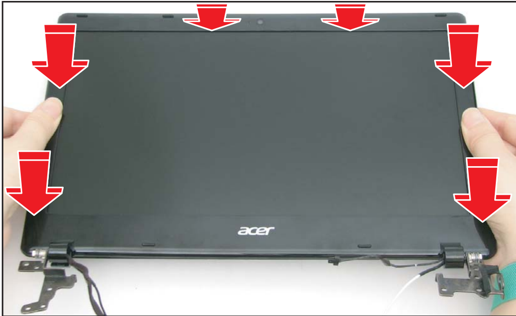
Figure 5:107. Installing the LCD Bezel (3 of 3)
