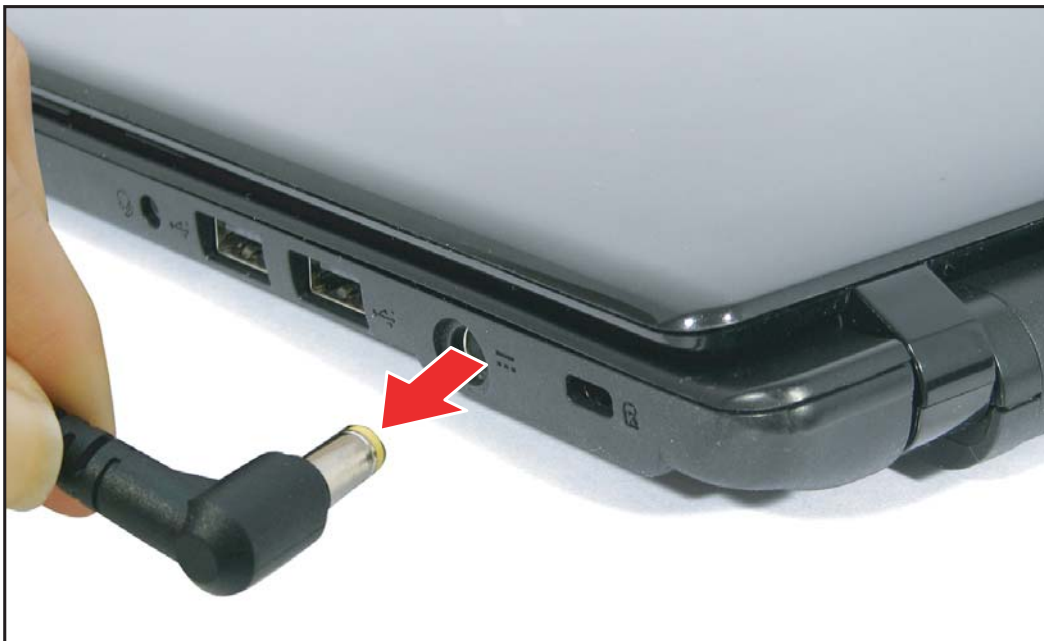
Figure 5:3. Disconnecting the Power Adapter
