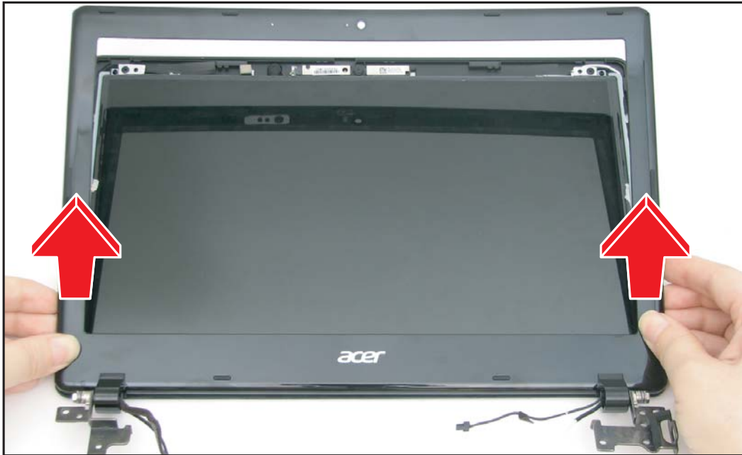
Figure 5:104. Removing the LCD Bezel (3 of 3)
