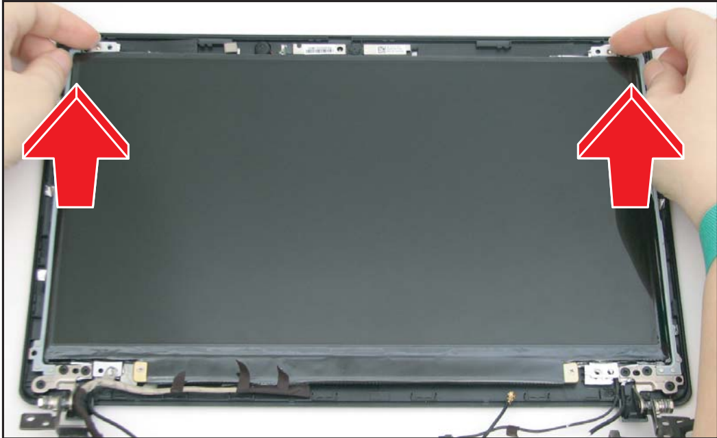
Figure 5:110. Removing the LCD Panel
