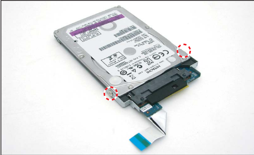
Figure 5:22. Installing the HDD Bracket
