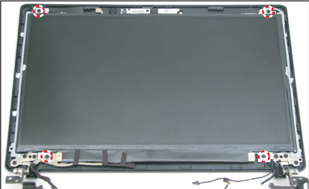
Figure 5:123. Securing the LCD Panel Screws
