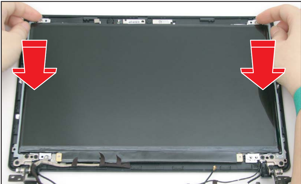
Figure 5:121. Installing the LCD Panel
