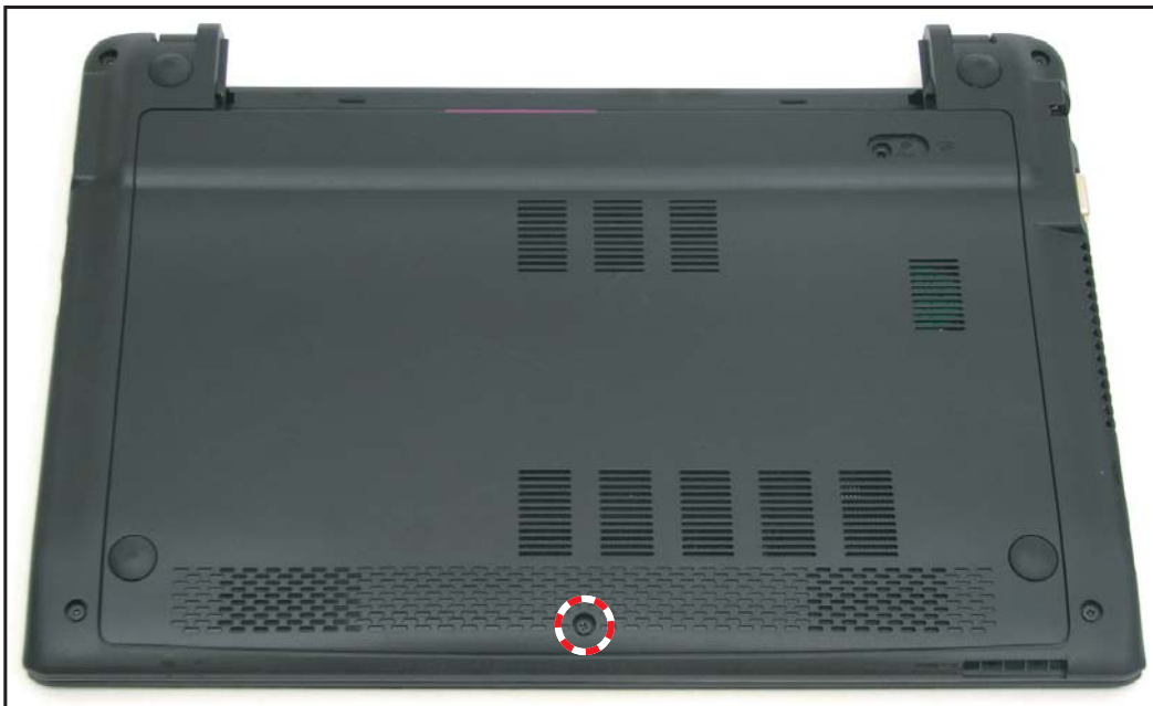
Figure 5:12. Securing the Base Door Screw
