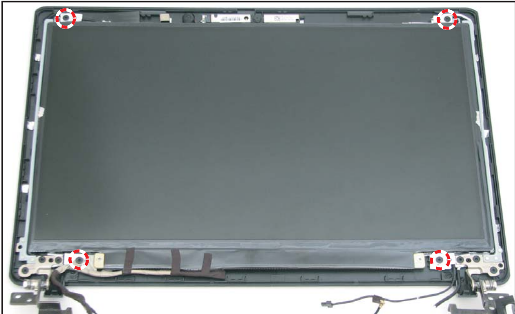
Figure 5:108. Removing the LCD Panel Screws
