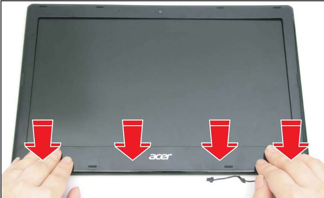
Figure 5:106. Installing the LCD Bezel (2 of 3)
