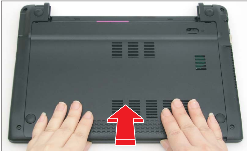
Figure 5:11. Installing the Base Door
