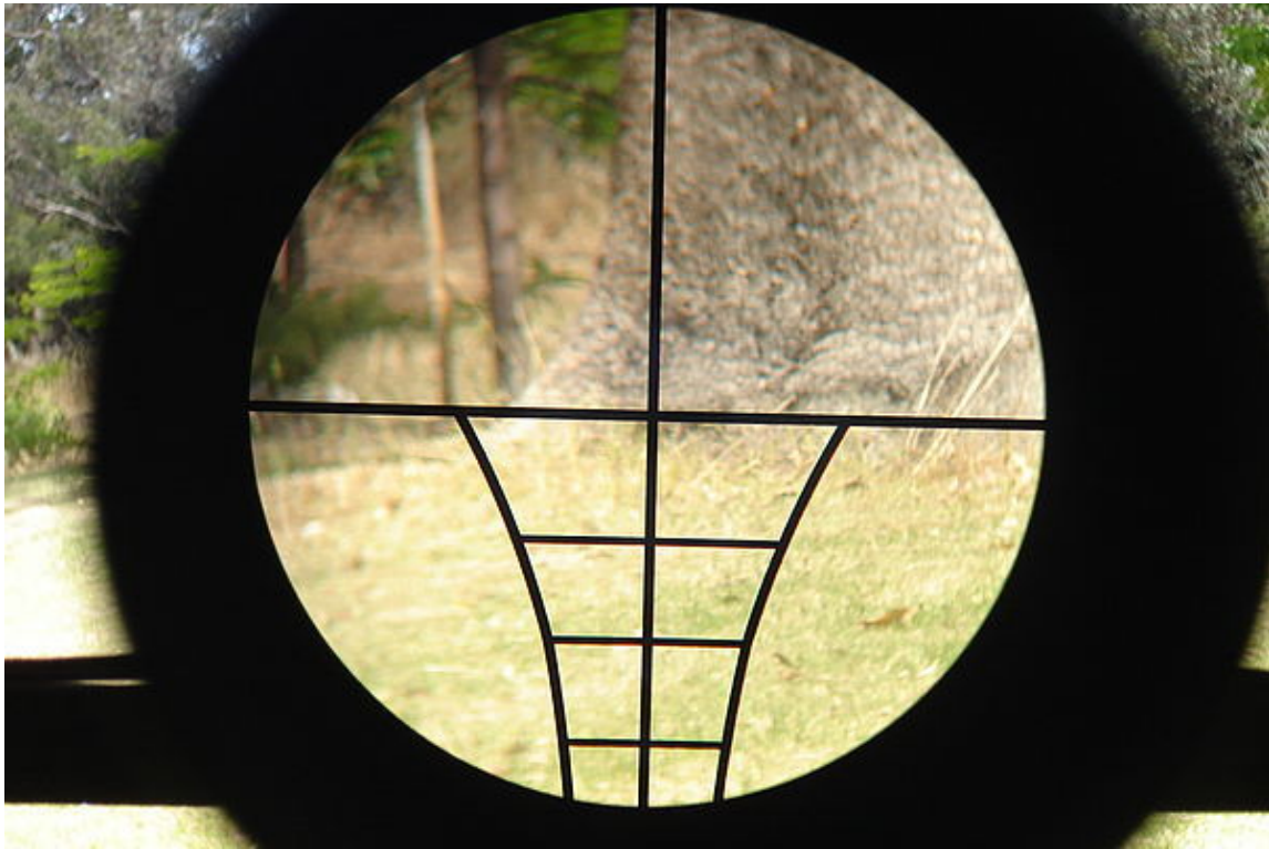
The reticle of a modern crossbow telescopic sight allows the shooter to adjust for different ranges
