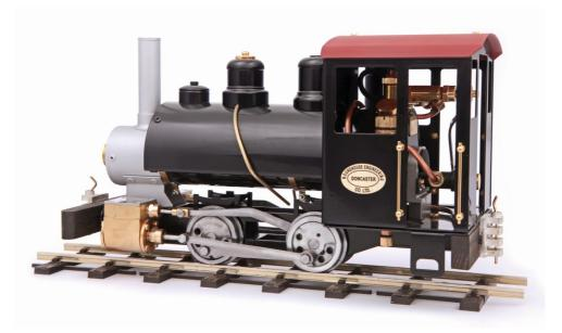
'Sammie' is the second locomotive in our 'basic Series'. Offered in a ready to run form as illustrated above, this simple, slip-eccentric, internally gas fired model can be easily enhanced using our accessory packs.
