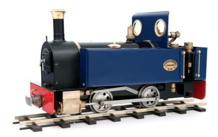
'Millie' was the first of our range of low cost locomotives. This simple, slip-eccentric, externally gas fired model can be easily enhanced with a number of separately available accessory packs.
