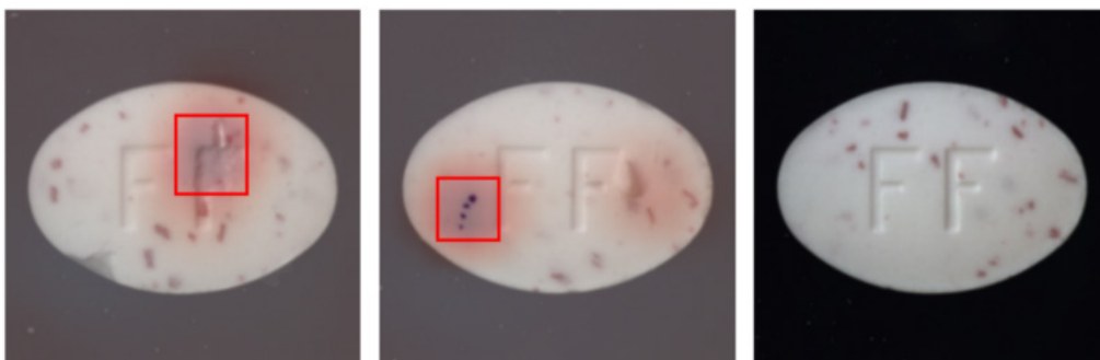
Figure 5. Model deployed to identify anomalous (the first two images) and normal (the image on the right) pills.
