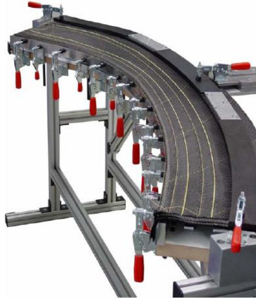
図 1.4.1 (3) - 3 Assembling of carbon fiber component from the aerospace < Application areas of one-side stitching technique ALTIN Nähtechnik GmbH >
