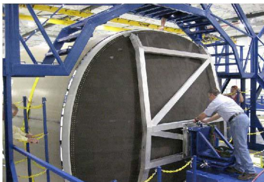
図 1.4.3 (1) - 3 B787 Aft Pressure Bulk Head
