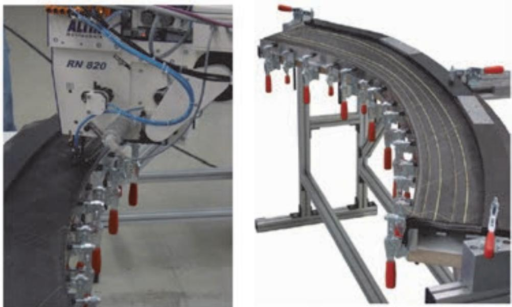
図 1.4.1 (3) – 3 Assembling of carbon fiber component from the aerospace
