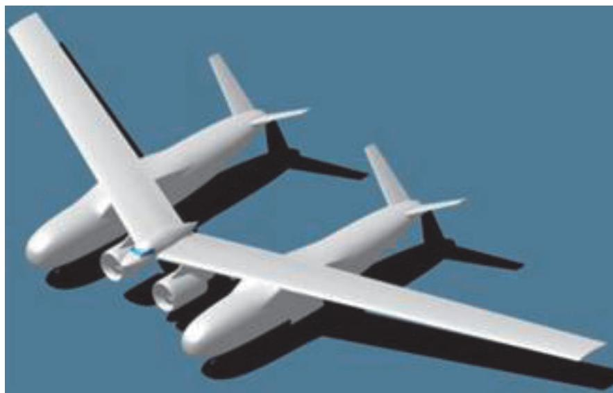
図 2.1.1 (3) – 2A 双胴機–Northrop Grumman
