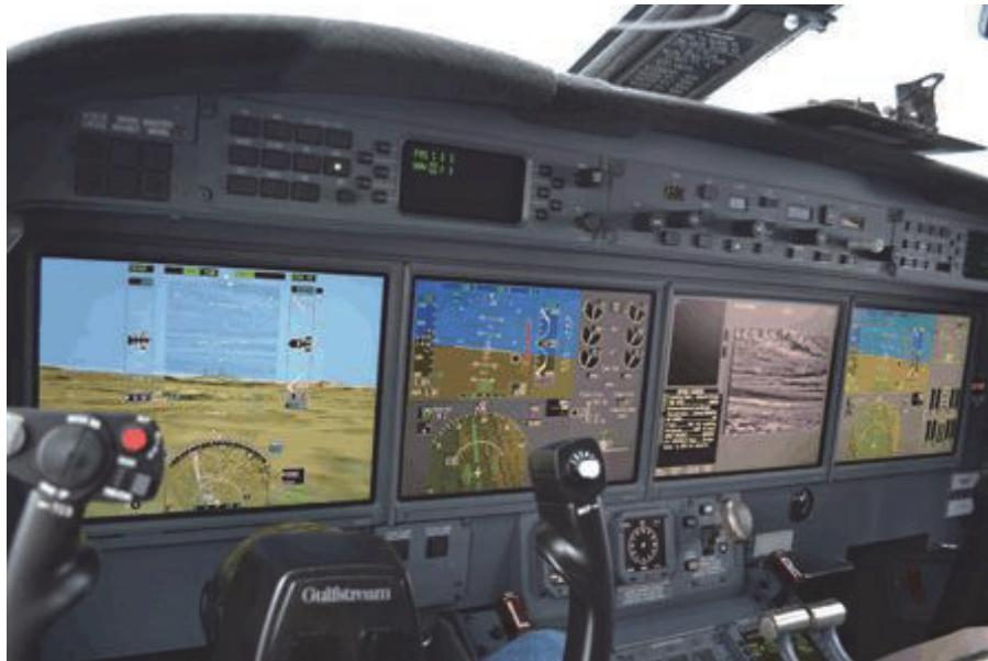
図 2.2.2 (2) – 1 Honeywell 社の Synthetic Vision
