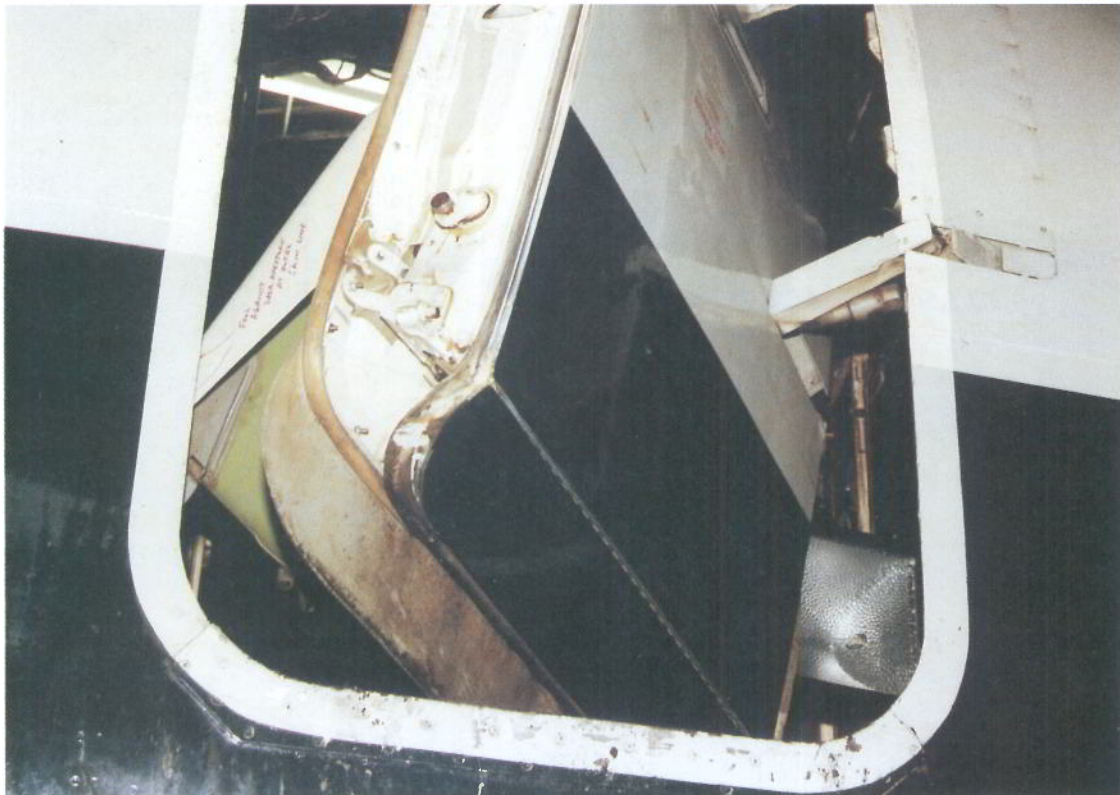
b - Door Position With Witness Marks Aligned-External
