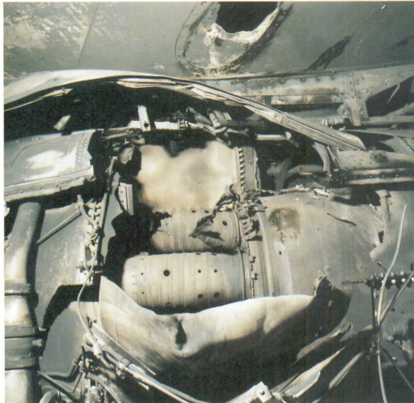
Engine rupture and holed fuel tank access panel
