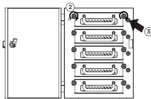
2. Tighten two hand screws to secure HDD tray
