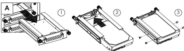
A. Installing 3.5" Hard Drive with Standard Tray
