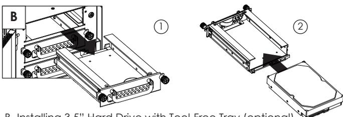
B. Installing 3.5" Hard Drive with Tool-Free Tray (optional)
