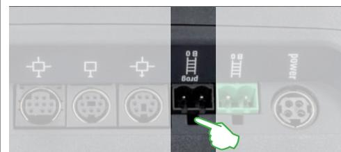
The programming track may not have any direct electrical contact with the layout and no other users (examples: lighting, turnout decoders, lighted track bumpers, etc.) may be connected to it. The programming track required to read, program, and edit locomotives and powered units in the DCC or Motorola (MM2) formats. No programming track is needed for registering mfx locomotives.
