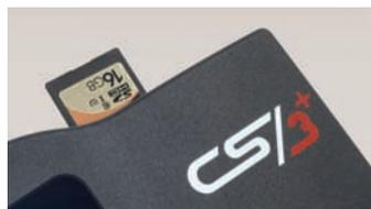
With an SD card (SDHC), you can expand the internal memory (4 GB) by up to 32 GB of memory. All you have to do is plug the card in the card slot. You do not have to do any other settings.
