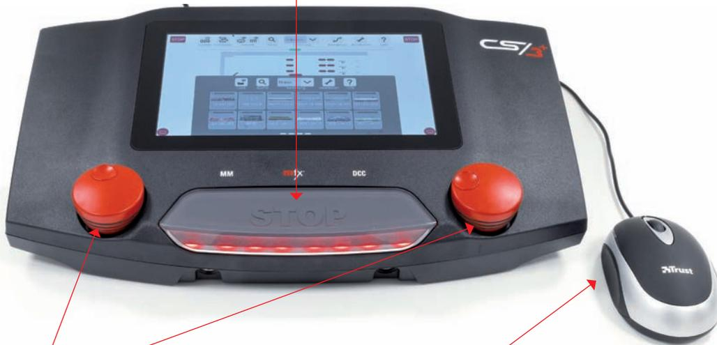
The control knobs are used to control the speed of locomotives (placed in the side locomotive controllers). Pressing on a control knob changes the direction of travel for the locomotive being controlled.
