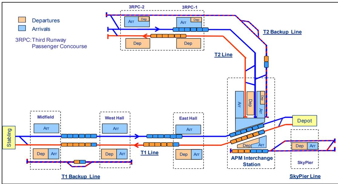
5.85 HKIA needs an APM fleet size of 110 cars to bring its annual handling capacity to 100 million passengers by 2030. It is recommended that the existing APM depot underneath T2 be relocated underground east of T2. This will be sized to accommodate the ultimate APM network capacity but can be constructed in stages.
