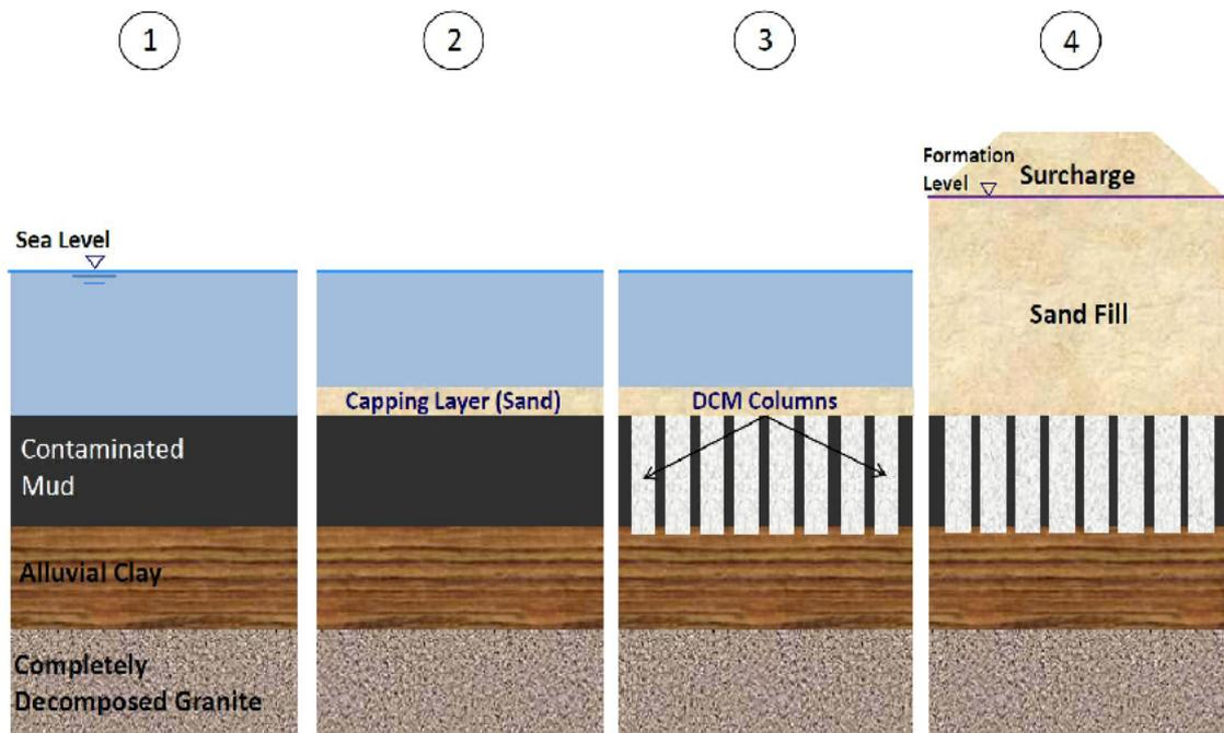
5.65 Sand fill compacted by vibro-compaction is proposed as the key fill material for the reclamation. In all areas, surcharge preloading is proposed to control the anticipated settlement during the service life of the landfill. The duration of surcharge preloading will depend on the results of instrumentation monitoring throughout construction but is anticipated to be in the range of 4 to 12 months.
