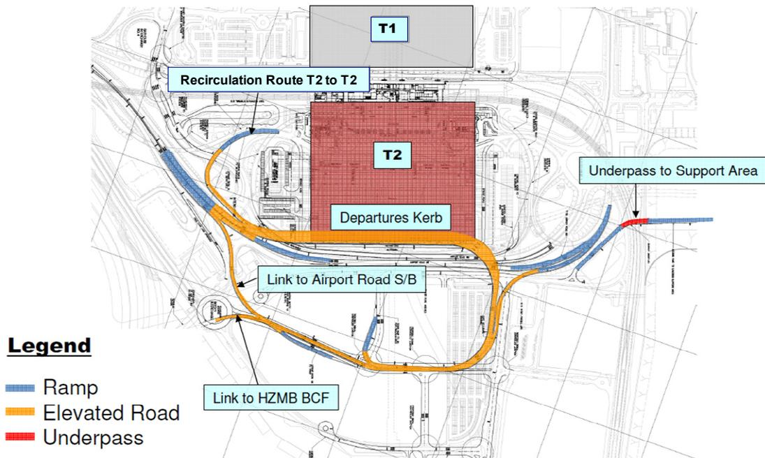
Figure 5.25 : Road Connection to and from the Airport via HKBCF/TMCLKL for Three-Runway Option
