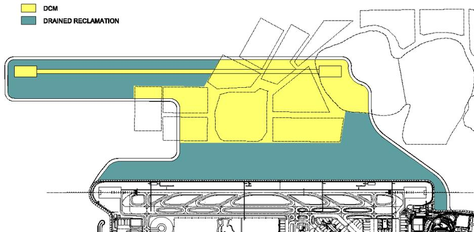
5.67 The approximate seabed level in the reclamation area is at -6 mPD<sup>59</sup> (see Figure 5.36). Assuming mean sea level at +2 mPD, the average water depth in the reclamation area will be 8m.
