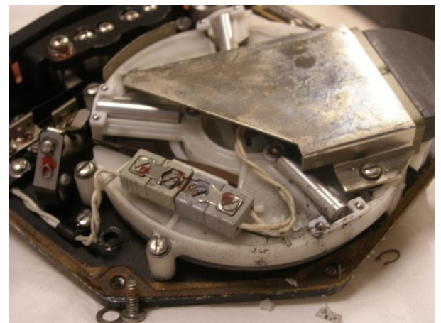
Picture 8: broken tape casing
