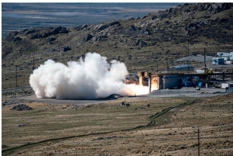
Static fire test of the first stage of the newly developed 34.5" common hypersonic missile
