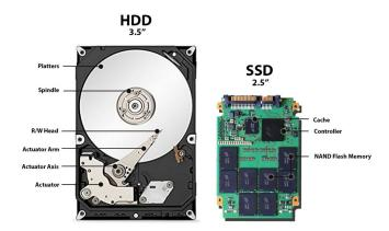
If you intend to wipe your whole HDD laptop, the process is rather straightforward. The data is written at a precise location on a magnetic (hard) platter (why it is called a hard drive) and your OS knows precisely where it is on the platter, where to delete it, and where to overwrite it for secure deletion using simple processes (like just overwriting that location over and over until no traces are left).
