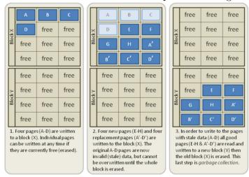
As you can see in the above illustration, data (from a file) will be written to the four first pages of Block X. Later new data will be written to the remaining pages and the data from the first files will be marked as invalid (for instance by a Trim operation when deleting a file). As explained on https://en.wikipedia.org/wiki/Trim\_(computing) [Wikiless] [Archive.org]; the erase operation can only be done on entire blocks (and not on single pages).
