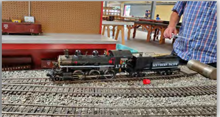
Larry's Accucraft Mogul 2-6-0 butane fired steam engine
