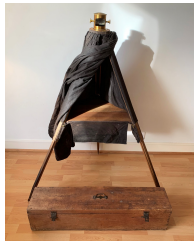
13. Camera Obscura Lacquered brass tube camera obscura with rotating meniscus prism, mounted on a walnut tripod with detachable drawing bench, dark cloth and original wooden case Labeled E. Mary & Filis, Paris FRONT COVER: LOUIS JACQUES MANDÉ DAGUERRE (French, 1787–1851) Fantaisie , circa 1827. Dessin-fumée, 7,9 x 6,1 cm BACK COVER: WILLIAM HENRY FOX TALBOT (English, 1800–1877) Leaf study , probably 1841. Photogenic drawing negative, 21,9 x 18,6 cm
