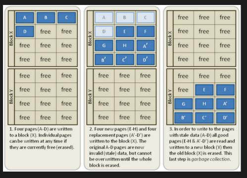
As you can see in the above illustration, data (from a file) will be written to the four first pages of Block X. Later new data will be written to the remaining pages and the data from the first files will be marked as invalid (for instance by a Trim operation when deleting a file). As explained on https://en.wikipedia.org/wiki/Trim\_(computing) <sup>[Wikiless]</sup> [Archive org]; the erase operation can only be done on entire blocks (and not on single pages).
