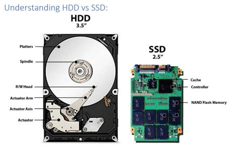
If you intend to wipe your whole HDD laptop, the process is rather straightforward. The data is written at a precise location on a magnetic (hard) platter (why it is called a hard drive) and your OS knows precisely where it is on the platter, where to delete it, and where to overwrite it for secure deletion using simple processes (like just overwriting that location over and over until no traces are left).
