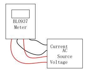
It is recommended to use the single-point calibration method, the accurate source provide the rated voltage U0(V), current I0(A) and active power P0(W) to the BL0937 meter. The corresponding pulse frequency U\_Freq0(Hz), I\_Freq0(Hz) and P\_Freq0(Hz) measured by MCU can be converted to the corresponding conversion coefficient:
