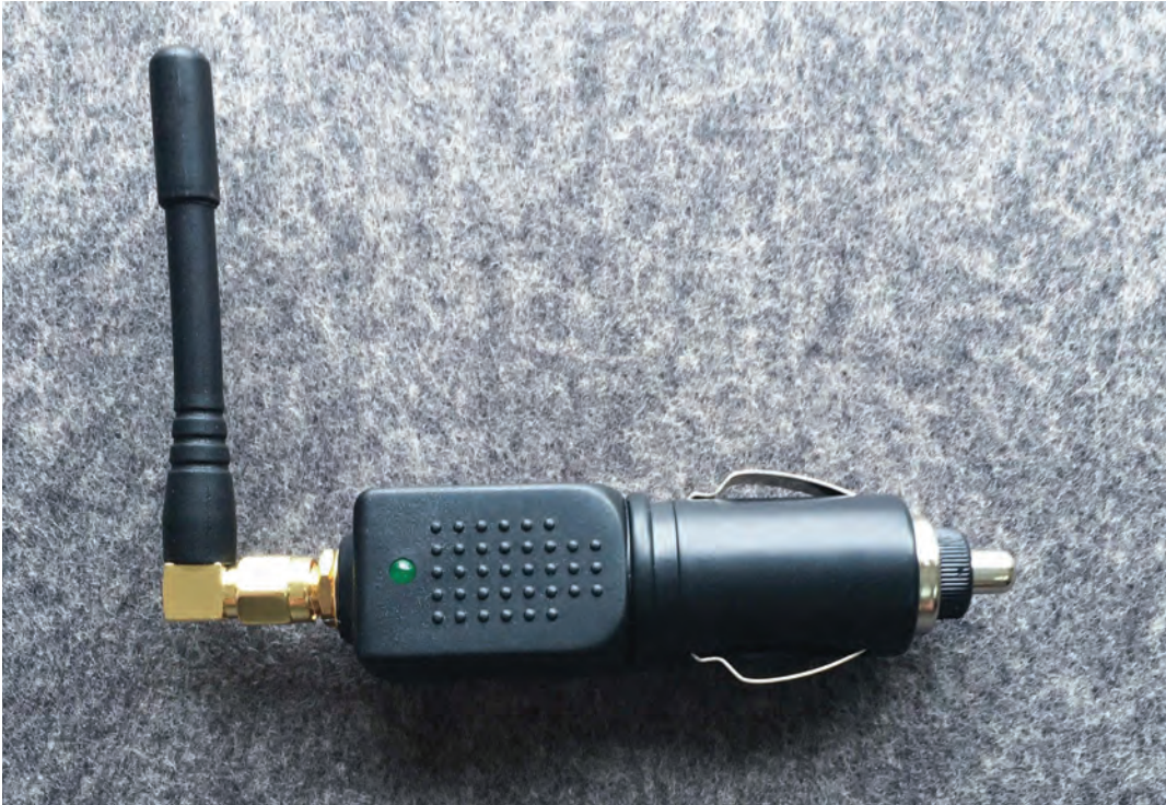
Example of a low-cost, commercially available GPS jammer
