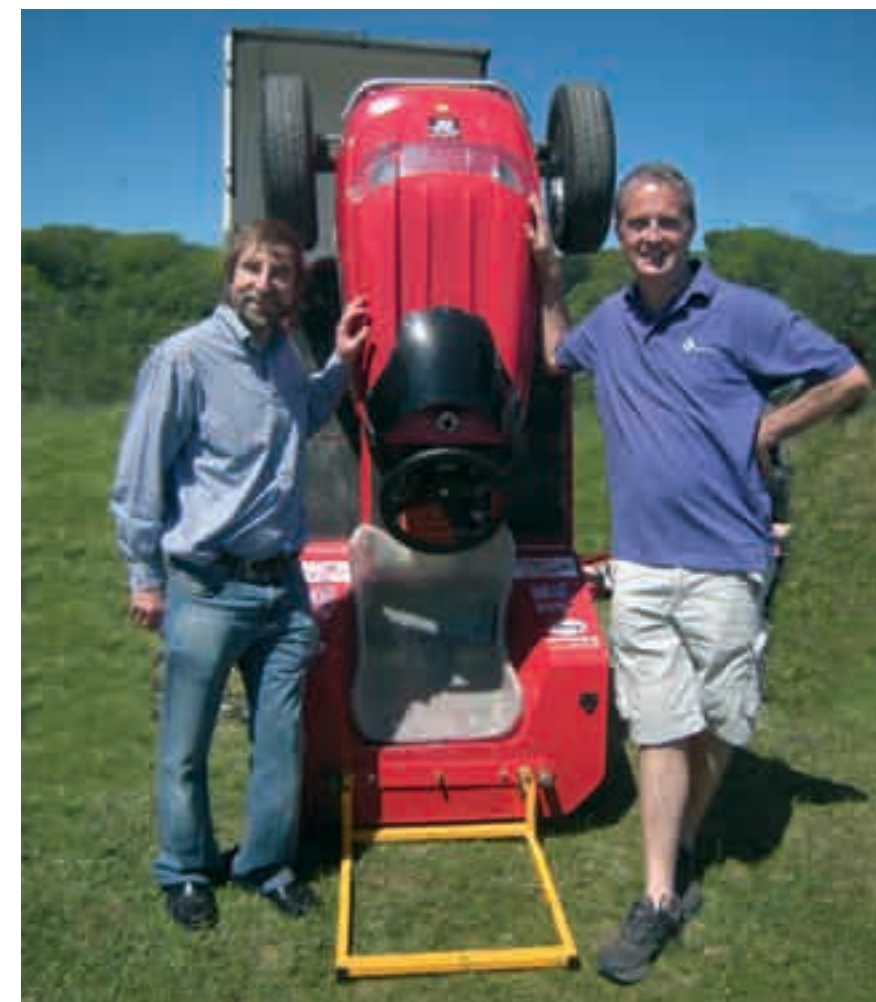
▲ Donald Wales (right) and author Brian Radam in 2010, with the world's then fastest lawnmower, a Countax A Series model assembled 90% from standard Countax components and powered by a 999cc Kawasaki FX1000V twin-cylinder engine and cutter deck – truly a cut above the rest. Don holds nine UK land-speed records.
