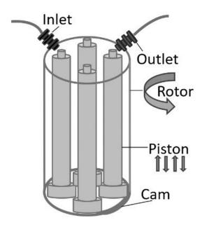
**FIGURE 3:** Schematic of milliGAT pump functioning (image credit: author).
