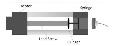
FIGURE 2: Schematic of infusion syringe pump (image credit: author).
