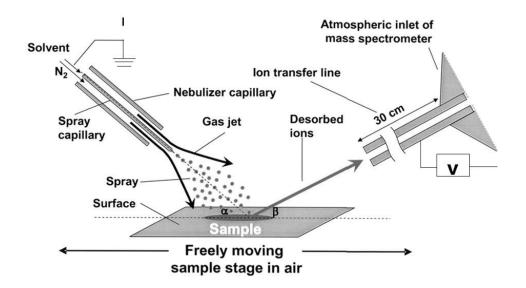
**FIGURE 1.** Diagram of desorption electrospray ionization platform setup, where  $\alpha$  is the incident angle (spray needle to surface) and  $\beta$  is the collection angle (surface to mass spectrometer inlet)<sup>3</sup>.
