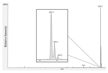
FIGURE 4: Example of extracted mass spectrum of rhodamine 6G.
