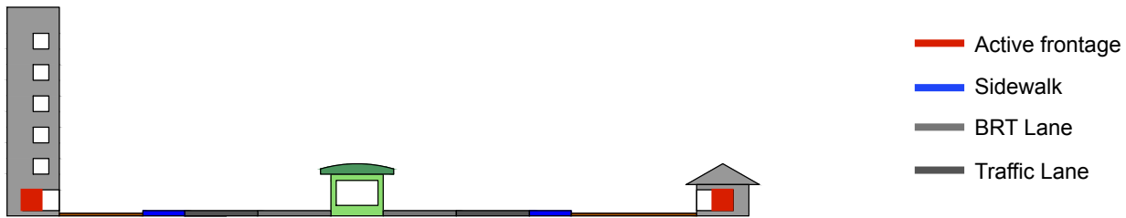
Figure 54: Cross-section of Station Type S5. Note the large building setback beyond the sidewalk.
