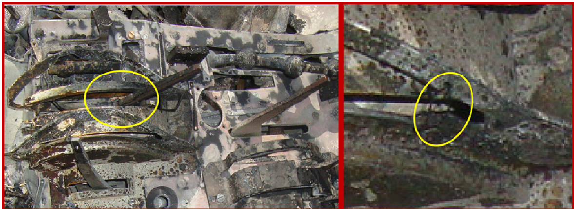
Figure 21 – Inviolable seal of the right engine power control lever.
