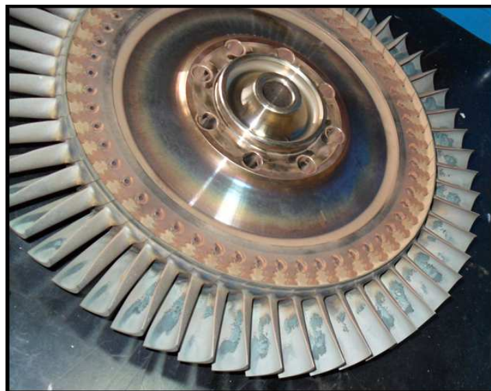
Figure 4 - Compressor turbine disk removed on account of corrosion at high temperatures.
