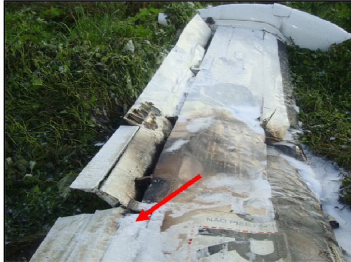
Figure 20 – Left wing flap 18-degree deflection (the same as the one of right wing).
