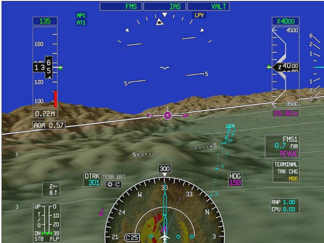
Figure 22: Gulfstream PFD AoA Located Under Airspeed Tape (Gulfstream, 2003)
