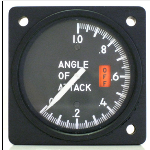
Figure 8: Teledyne Avionics Angle of Attack Indicator (Starfleet Support, LLC, nd)
