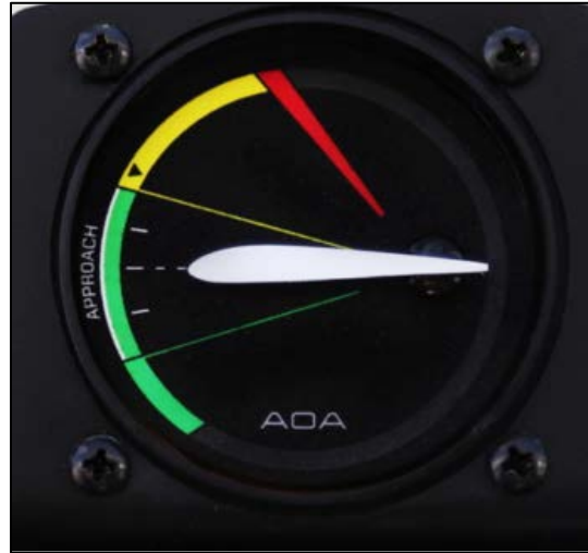
Figure 28: ICON A5 Light Sport Aircraft AoA indicator (ICON, 2013)
