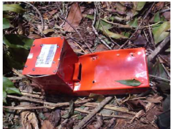
Figure 20: Base of the SSCVR unit, PR-GTD
