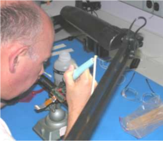
Figure 23: Flat cable recovery, PR-GTD SSCVR
