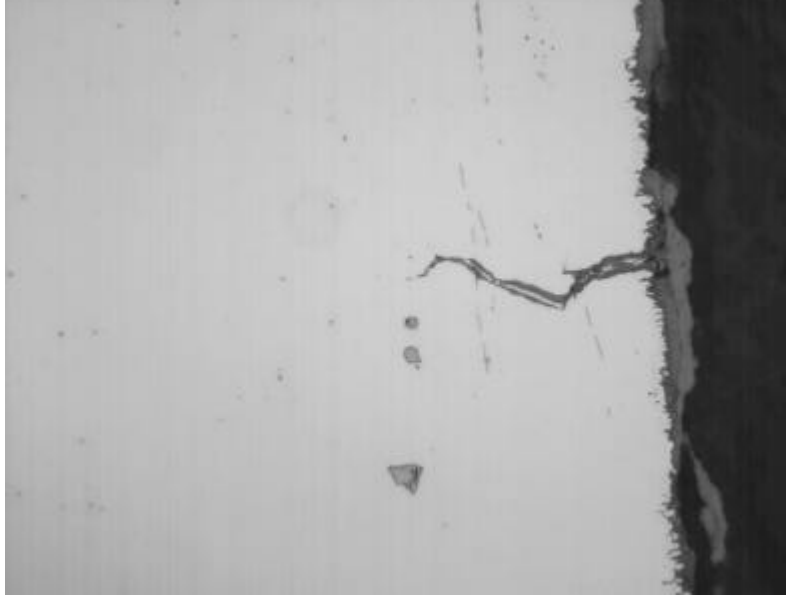
Figure C11. Secondary intergranular crack on aft face (right side)
