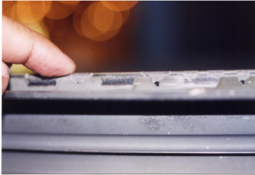
Figure B9. 5 th stage inner airseal cooling air holes - three holes partially opened
