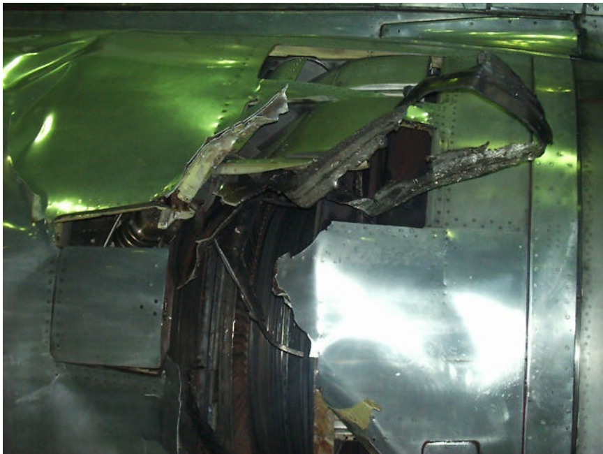
Figure A2. Damage on Engine #2 casing (2)
