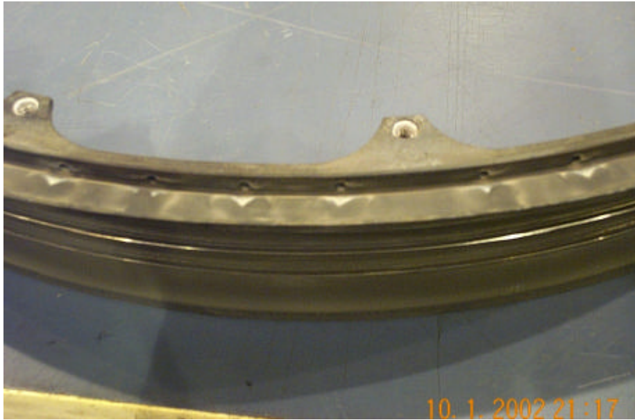
Figure B11. 4 th stage inner airseal - discoloration due to cooling air passing through cooling air holes, not found on 5 th stage inner airseal
