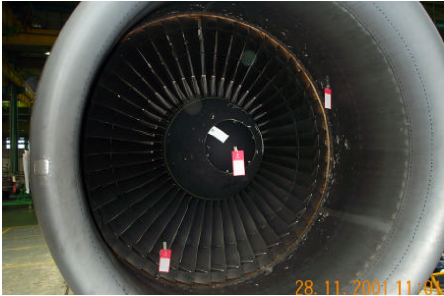
Figure A11. FOD on Engine #1 fan (1) - tagged debris
