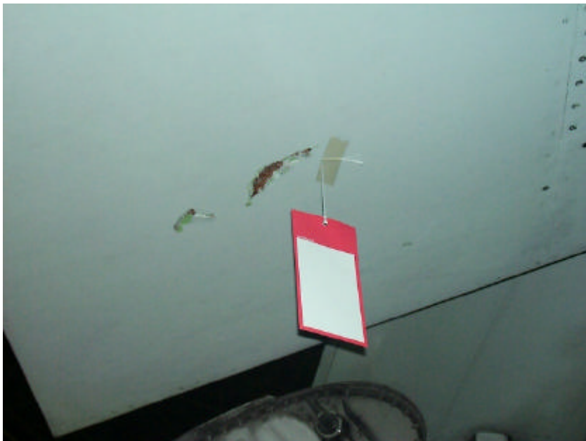
Figure A20. Damage on LH low speed aileron - tagged debris
