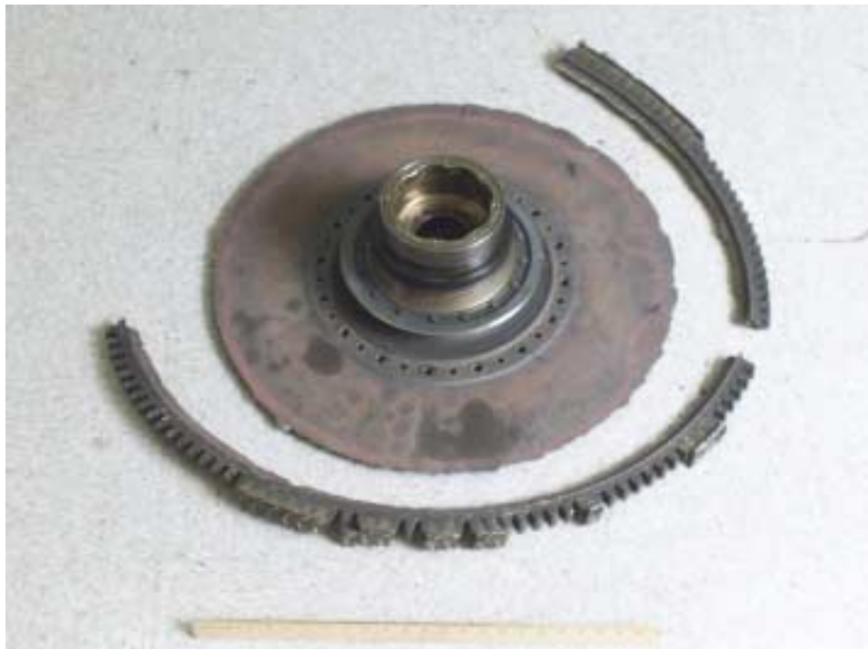
Figure 2. As-received disk that fractured all around the web. The two rim pieces were positioned next to the web portion as if intact.
