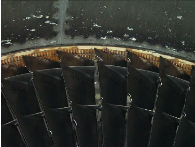
Figure A13. FOD on Engine #1 Fan/Fan Blades (2)
