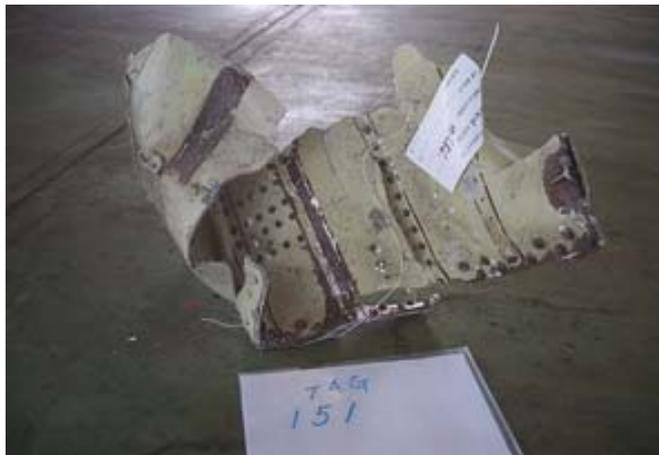
Figure 1.12-8 Wing trailing edge structure
