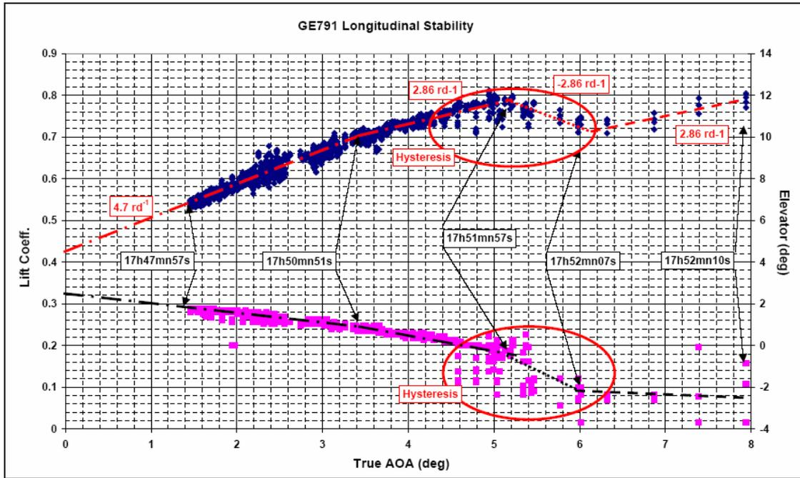
Figure 2.4-8 GE791 longitudinal stability (derived from FDR data)
