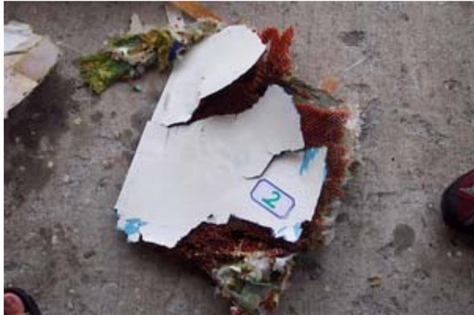
Figure 1.12-12 Vertical stabilizer honeycomb structure
