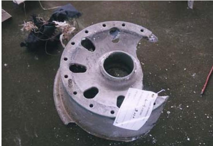
Figure 1.12-20 Broken wheel hub
