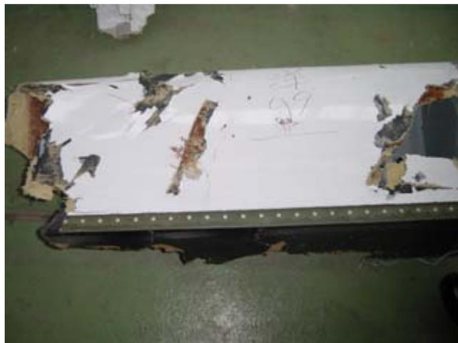
Figure 1.12-14 Rudder leading edge
