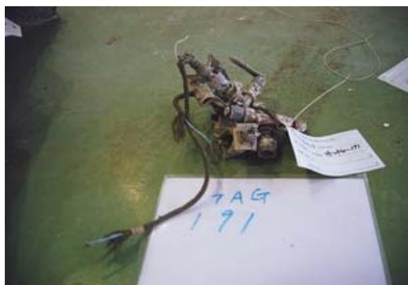
Figure 1.12-27 Wing de-icing regulator
