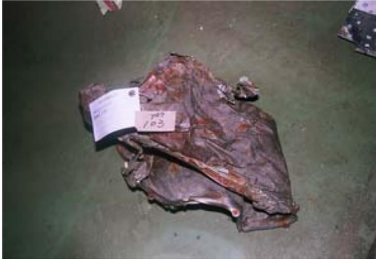
Figure 1.12-22 Exhaust pipe
