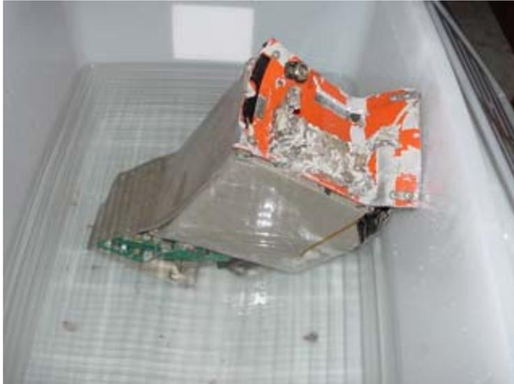
Figure 1.18-28 CVR closed view while recovered
