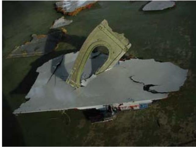
Figure 1.12-15 Window frame stuck into rudder
