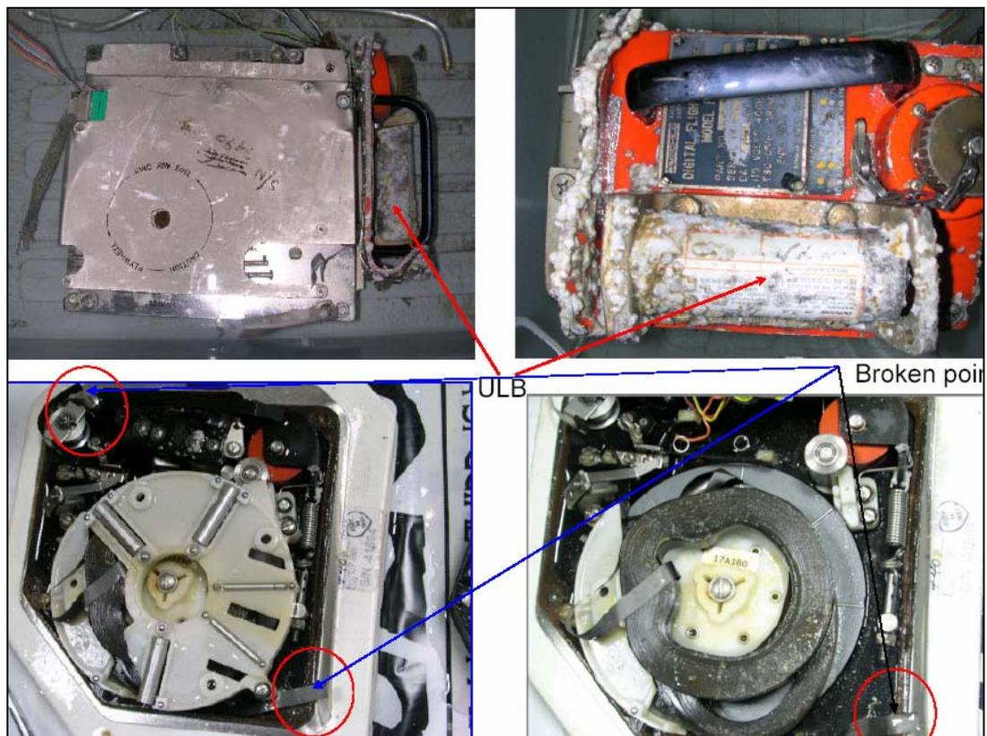
Figure 1.11-2 FDR physical damage and FDR tape
