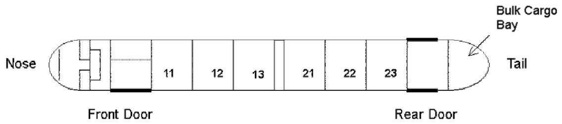
Figure 1.6-9 Schematics of ATR72 Cargo Bays
