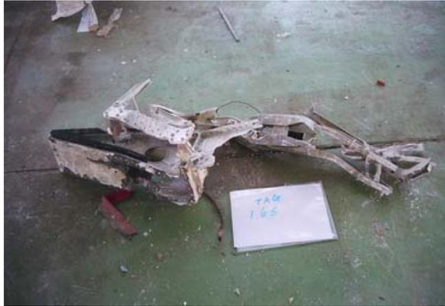
Figure 1.12-9 Flap driven mechanism
