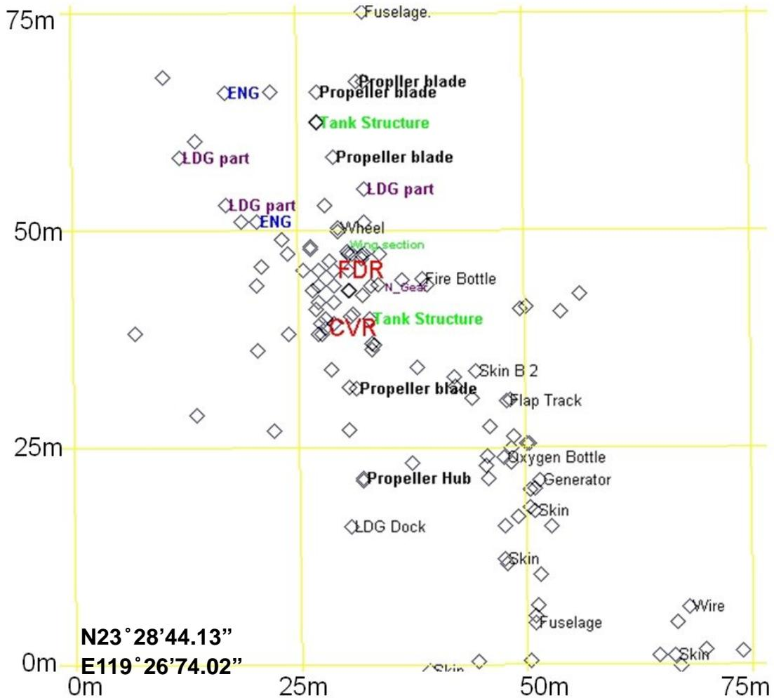
Figure 1.18-8 Wreckage distribution in dense area
