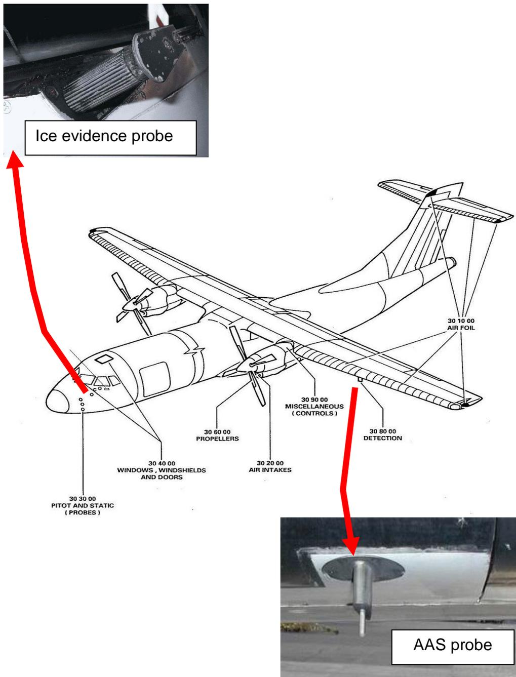
Figure 1.6-3 The Ice evidence probe & The Anti-Icing Advisory System (AAS) probe
