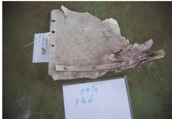
Figure 1.12-5 Cargo compartment partition
