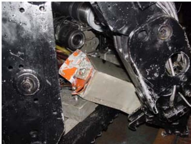
Figure 1.18-27 CVR recovered by ROV
