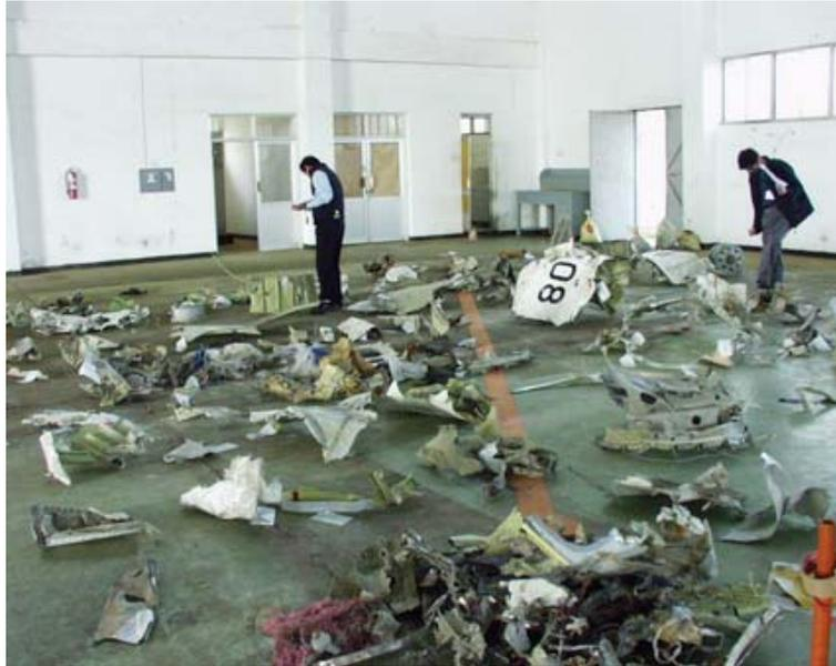
Figure 1.18-11 Underwater wreckage recovered by trawling operation
