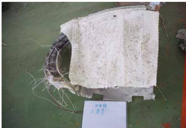
Figure 1.12-11 Flap leading edge structure
