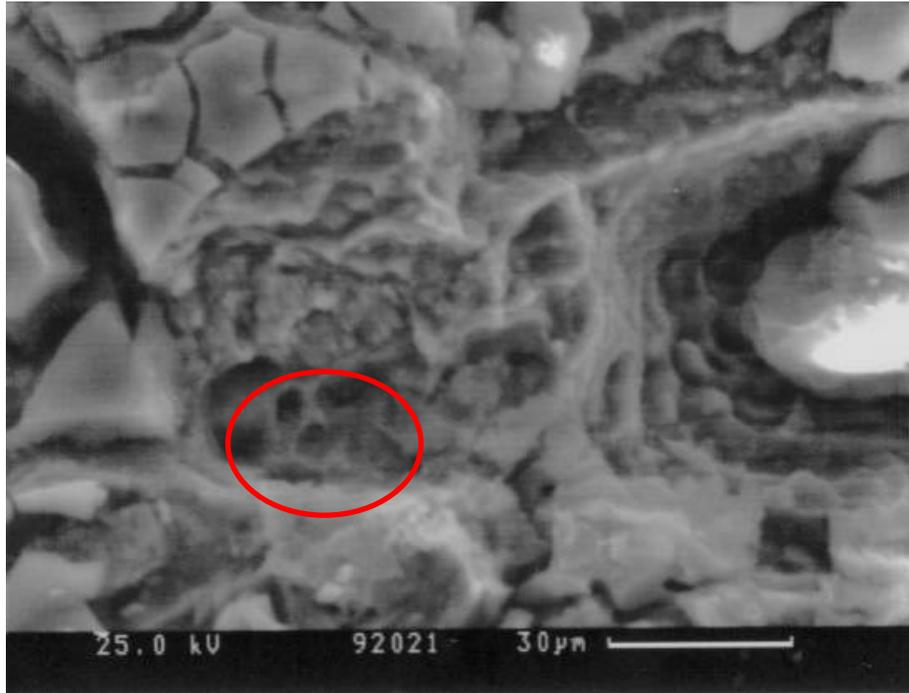
Figure 1.16-5 SEM examination showing the dimple structure (790X) ◦
