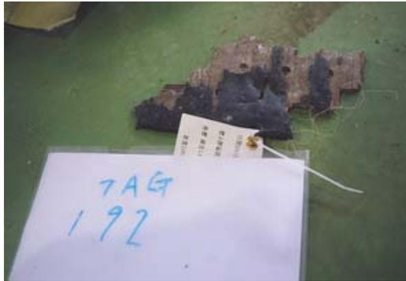
Figure 1.12-28 Wing de-icing boot
