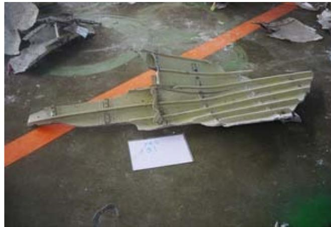
Figure 1.12-7 Wing tip structure (top of fuel tank)
