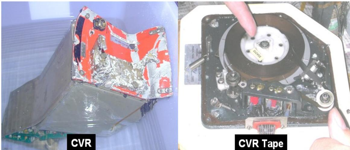
Figure 1.11-1 CVR physical damage and the CVR tape
