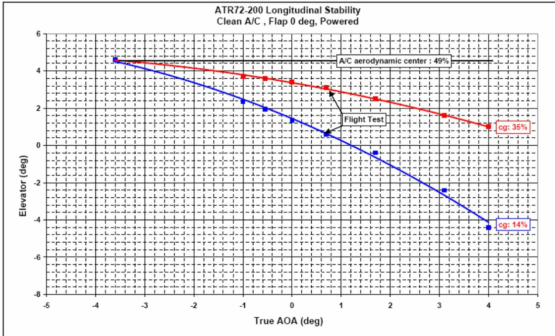
Figure 2.4-7 ATR 72-200 longitudinal stability
