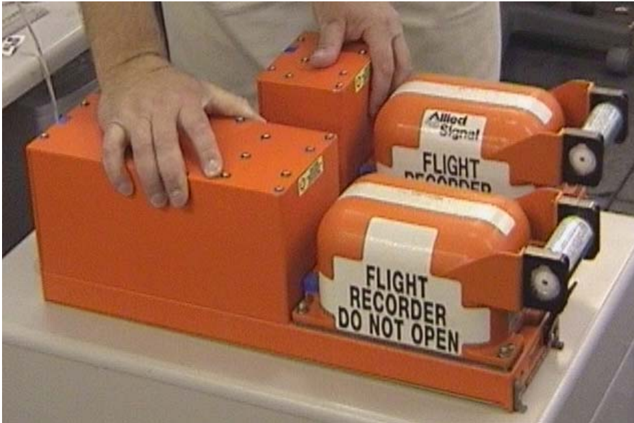
Figure 11.1 – Flight Data Recorder and Cockpit Voice Recorder
