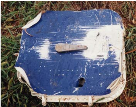
Figure 26.3 – Forward Equipment Centre Hatch
